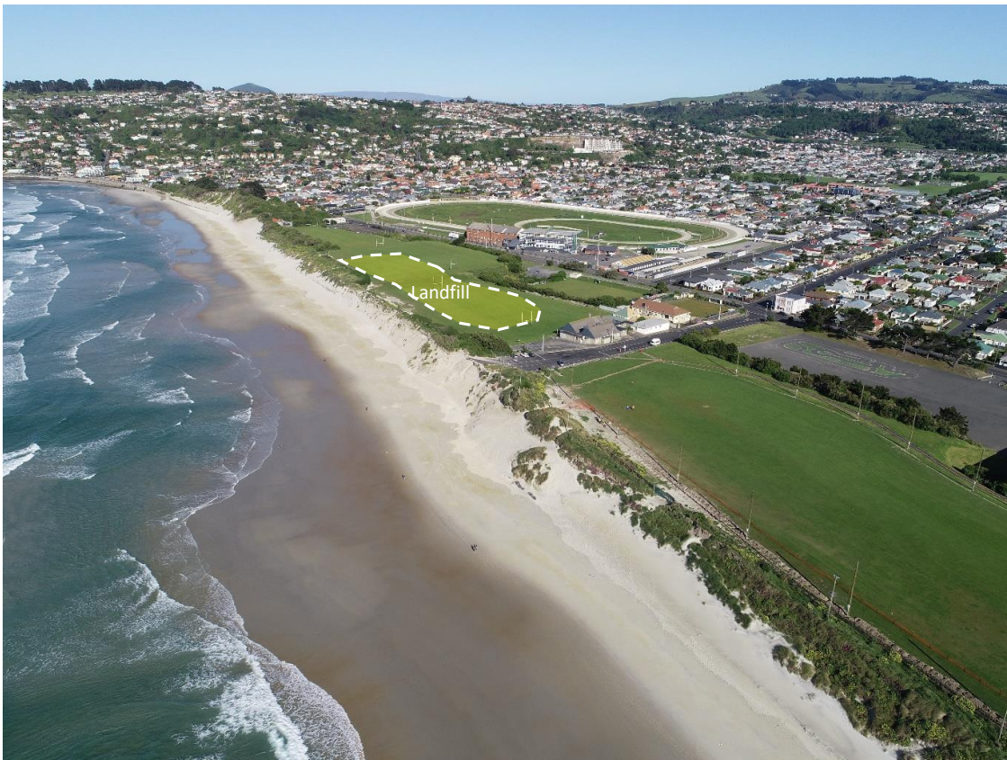
Figure A.4 View to the west from Moana Rua toward St Clair. Approximate area of historic landfill is outlined. DCC are currently investigating options to mitigate the potential impacts of sea level rise and projected erosion of the dune.
