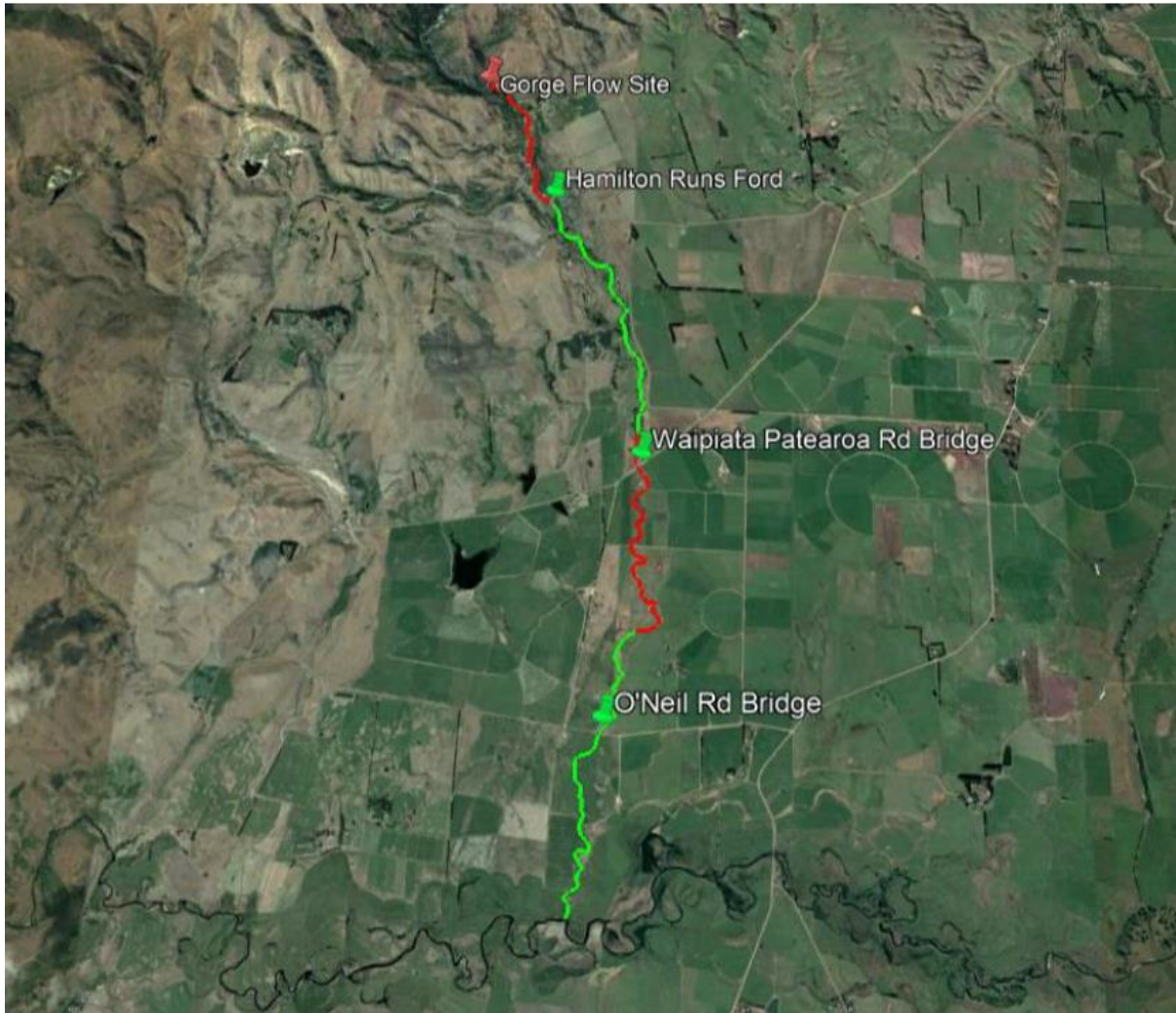
Figure 4: The gaining and losing reaches of the lower Pig Burn, red lines indicating losing reaches, and green lines gaining reaches (copied from Hickey 2020).
