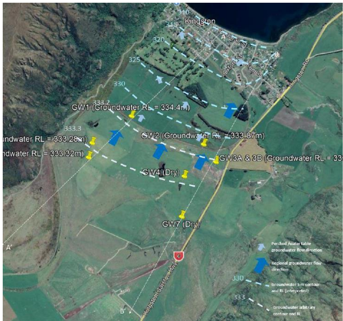
Figure 7. Conceptual hydrogeological flow model of groundwater beneath land treatment area (Source: Application)
