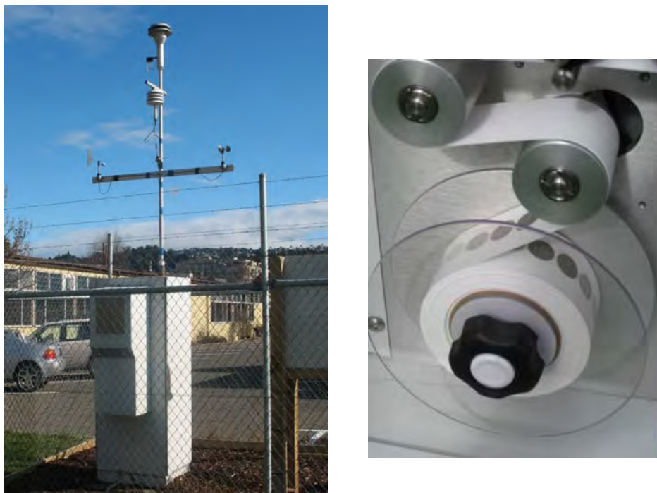
Figure 3 PM 10 and meteorology site in Central Dunedin and the filter tape a BAM1020 monitor; each filter tape spot represents one hour of sampled PM 10
