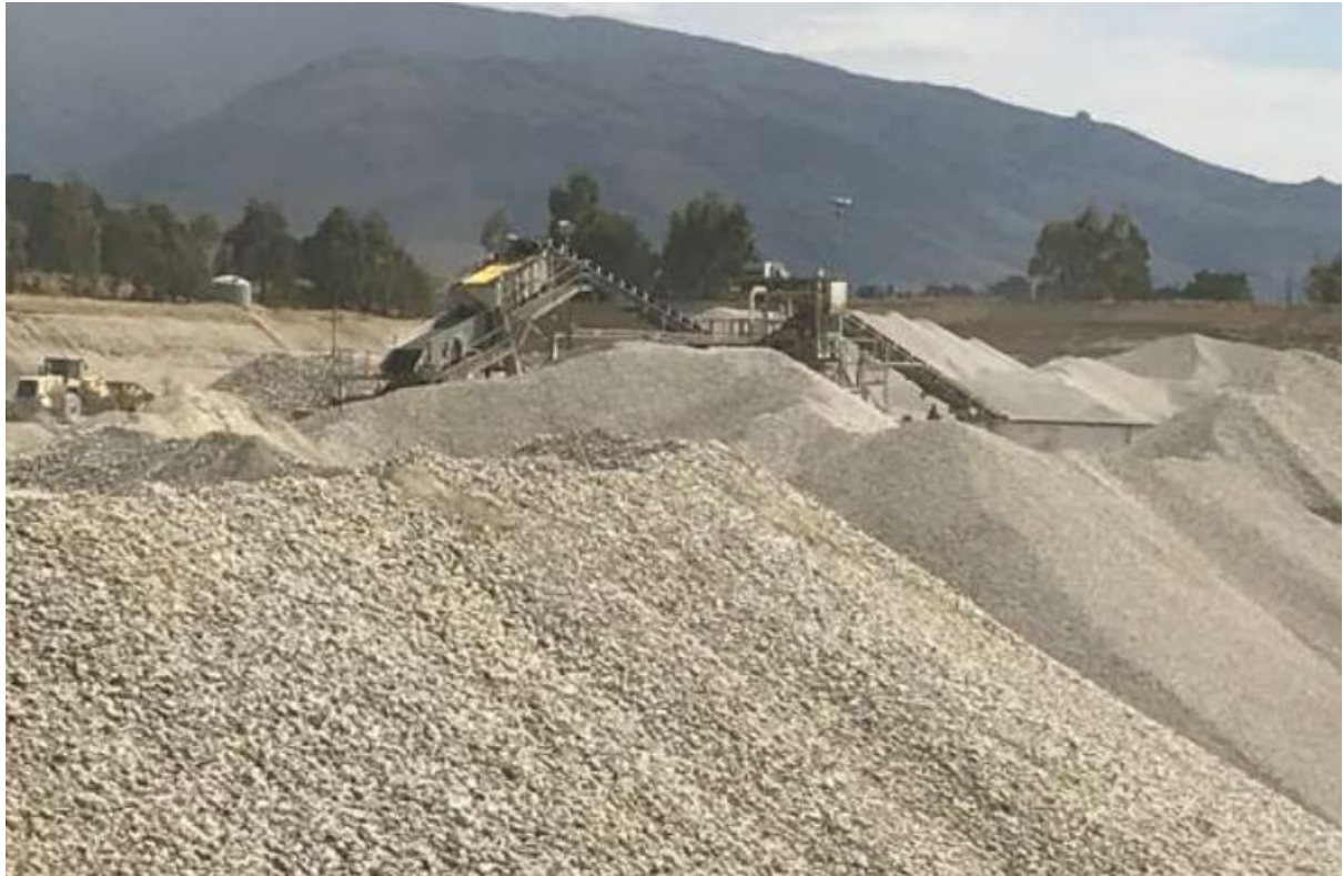
Figure 2. Photograph of screening and washing plant with washed aggregate in foreground (Source: Application)
