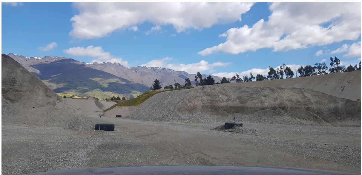
Figure 9. Photograph showing irrigation sprinklers and piles of aggregate. Processed aggregate and crusher plant are in the background
