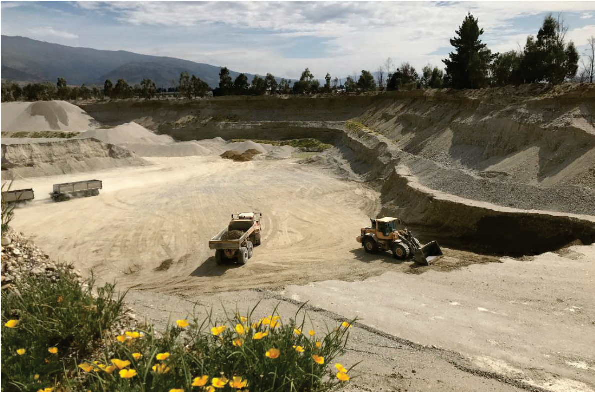
Figure 3-1 Photo of loader and trucks working on the quarry face (21/1/2020)
