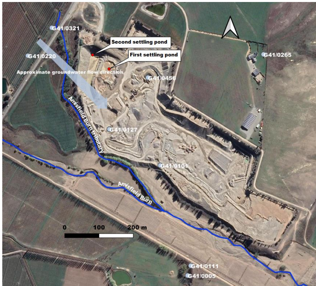
Figure 8: Location of settling ponds and bores
