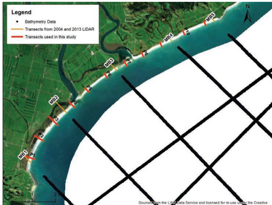
Figure 3.1: Location of ORC profile surveys (MB1-MB5), bathymetric transects, and beach profiles (P1-P11) created from 2020 Lidar used for this study.
