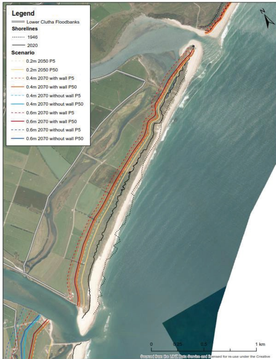
Figure 5: Koau to Matau Branches PFSP for P5 and P50 with and without training wall
