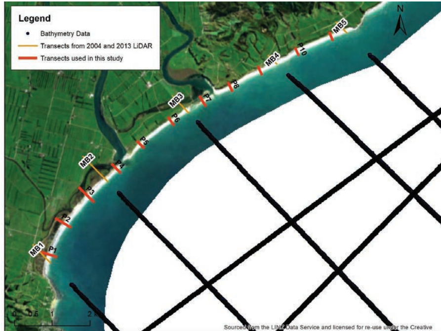
Figure 1: Location of ORC profile surveys (MB1-MB5), bathymetric transects, and beach profiles (P1-P11) created from 2020 Lidar used for this study
