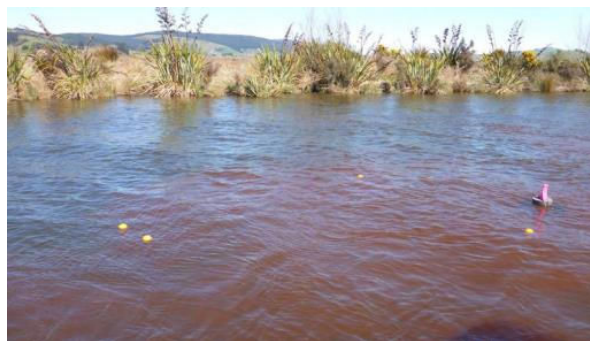
Figure 3.1.5 Drogue and oranges deployed within dye patch (12:43 PM).
