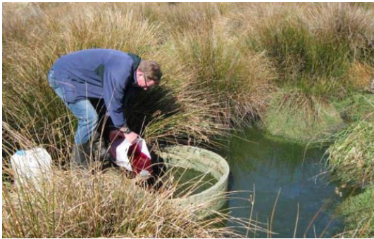
Figure 3.1.3 Dye being released at the intake to the outfall pipe
