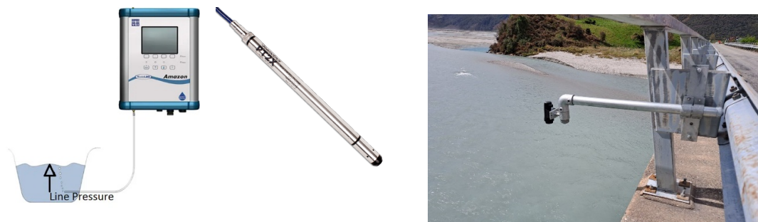
Fig. 4: Schematic of a bubbler system (YSI, on the left), pressure sensor/vented pressure transducer (middle, here Seametrics PT2X pressure and temperature sensor, also commonly used for groundwater applications), and a Waterwatch radar sensor mounted of the Dart River bridge (right).
