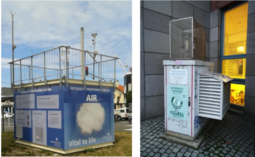
Fig. 13: Left: Wellington inner city air-quality monitoring portacom, which is also used as a display for public information. Right: inner city air-quality monitoring station in Gothenburg (Sweden) including gas measurements for Nitrous Oxides (NOx).
