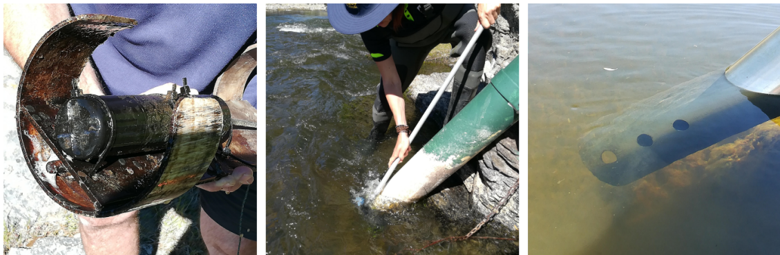
Fig. 10: Water quality sensors. Left: Oxygen sensor in mounting bracket during maintenance work (cleaning). Middle: manual cleaning of oxygen sensor installed in field. Right: field installation of water quality sensors in a protective steel tube.
