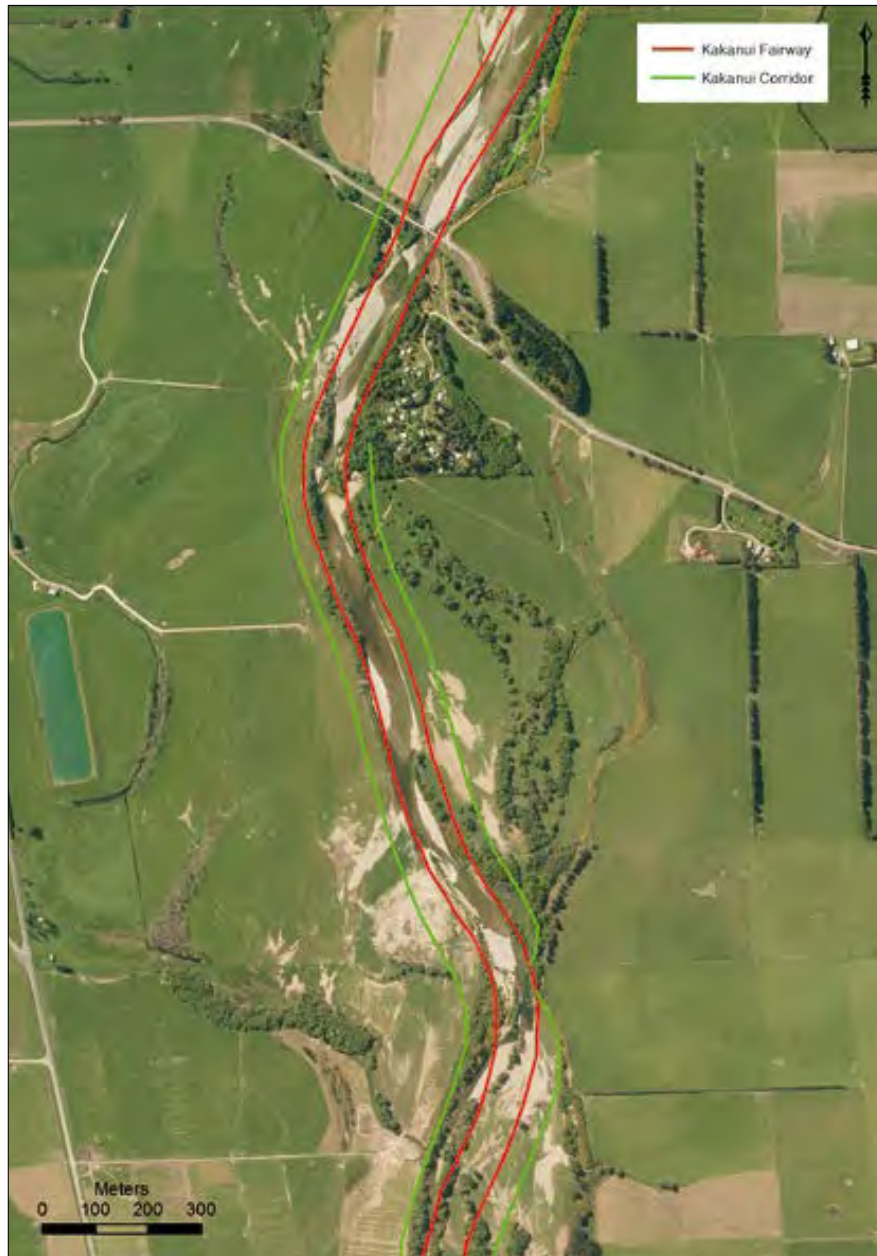
Figure 48. Kākaunui River fairway and corridor Map 6 (aerial photography collected in the summer of 2013/2014)
