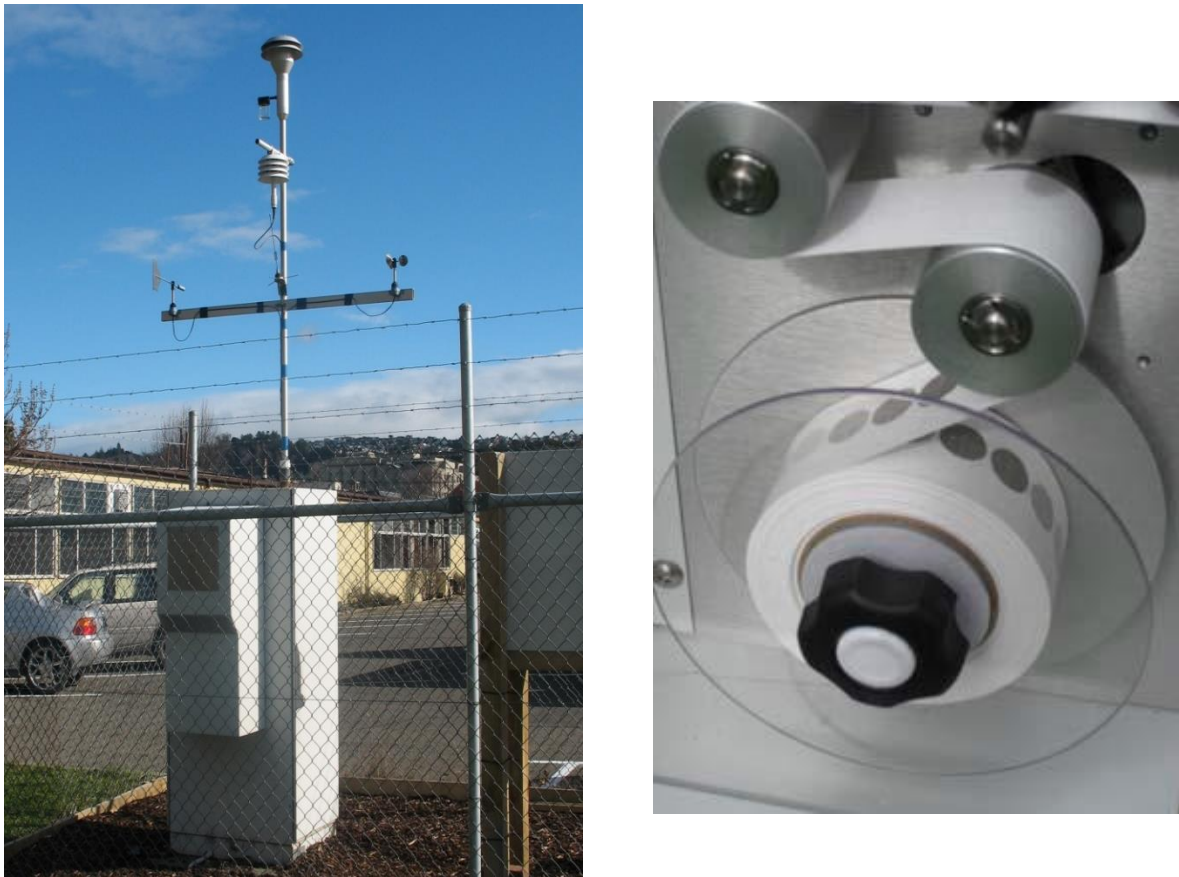
Figure 3 PM 10 and meteorology site in Central Dunedin and the filter tape of a BAM1020 monitor; each filter tape spot represents one hour of sampled PM 10
