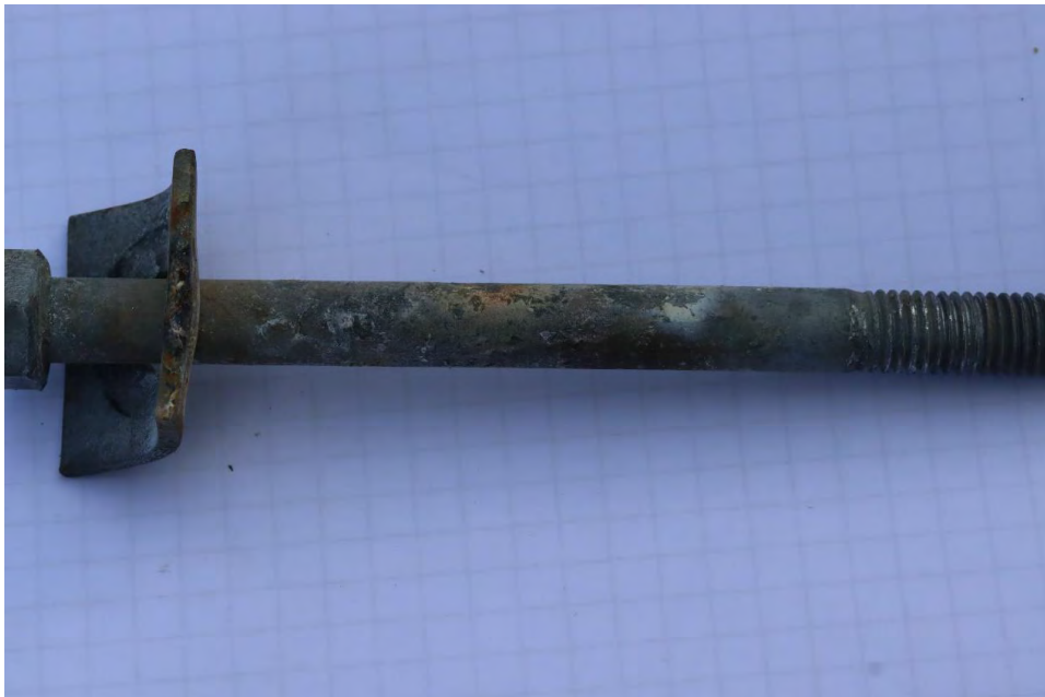
Fig. 77. Bolt from the centre of pole that held the metal stay arms with signs of heat damage. IMG_1440.JPG.
