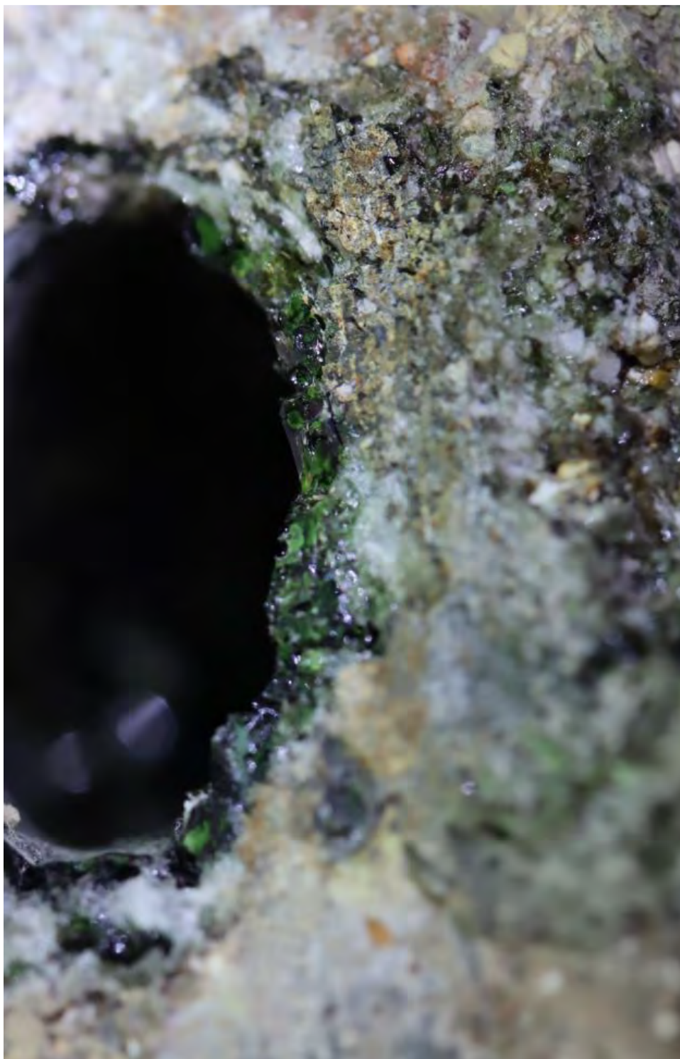
Fig. 74. Edge of hole and surface have appearance of melted glass.
