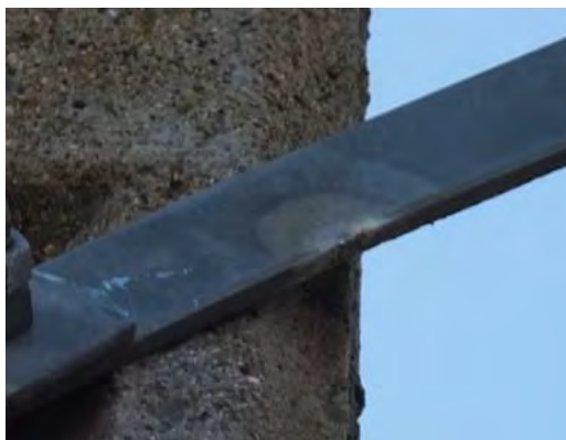
Fig. 45. Photograph (DSCF9361) above left identifies an arc mark to the lakeside metal stay arm on the upper section close to where it is secured to the wooden cross-arm with a double nut.
