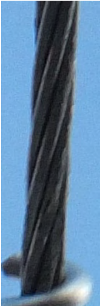
Fig. 50. Photograph (DSCF9362) to the left has been zoomed in and cropped, the strands appear to have a rough edge to them.
