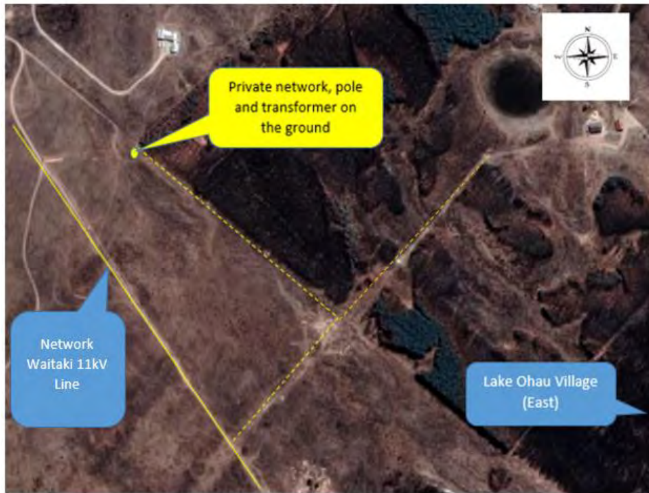
Fig. 4. Image above identifies Network Waitaki 11kV lines (solid yellow line) and the private network (dotted yellow lines). The Network Waitaki infrastructure was positioned along the maintenance track used to access the investigation start point.
