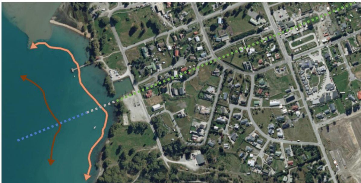
Figure 7.2: The mapped free face crest location and base locations along the edge of Lake Wakatipu around Glenorchy, together with the line along which the surface in Figure 7.1 is taken. The crest and base intersect at points D and E from that figure, respectively.
