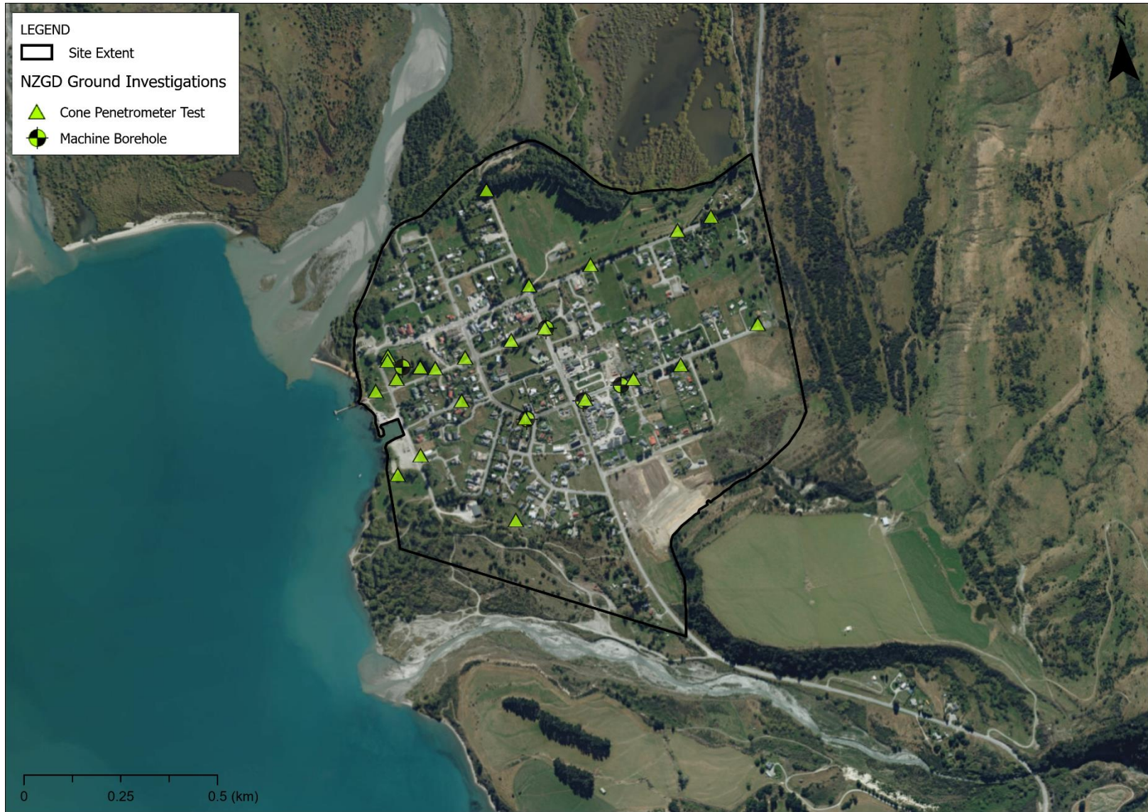
Figure 8.1: Geotechnical Investigation locations: data and logs available on the NZGD.
