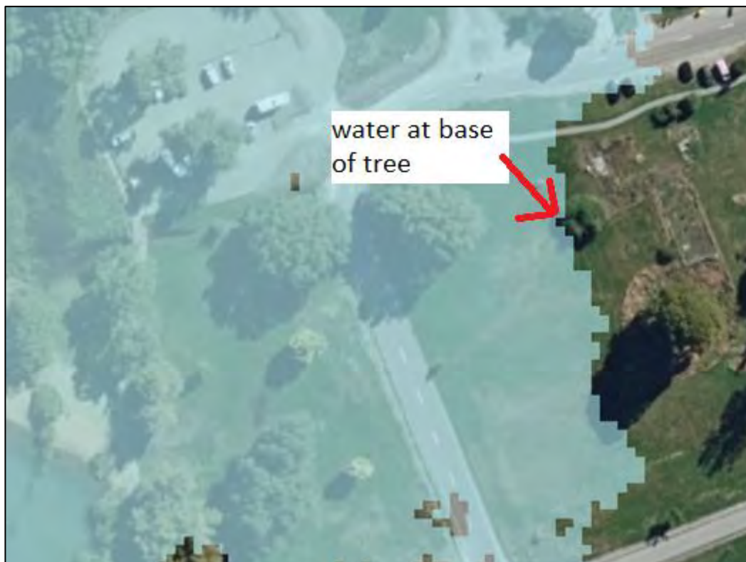
Figure 6-6 – Modelled flood extent in same location
