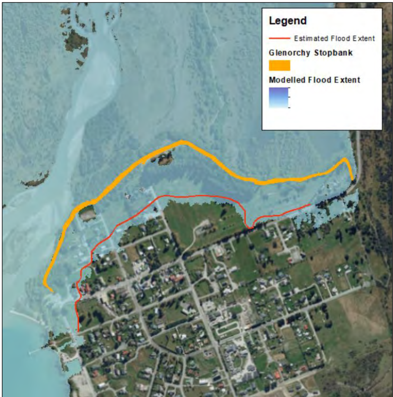
Figure 6-4 – Comparison of modelled flood extent with estimated actual extent
