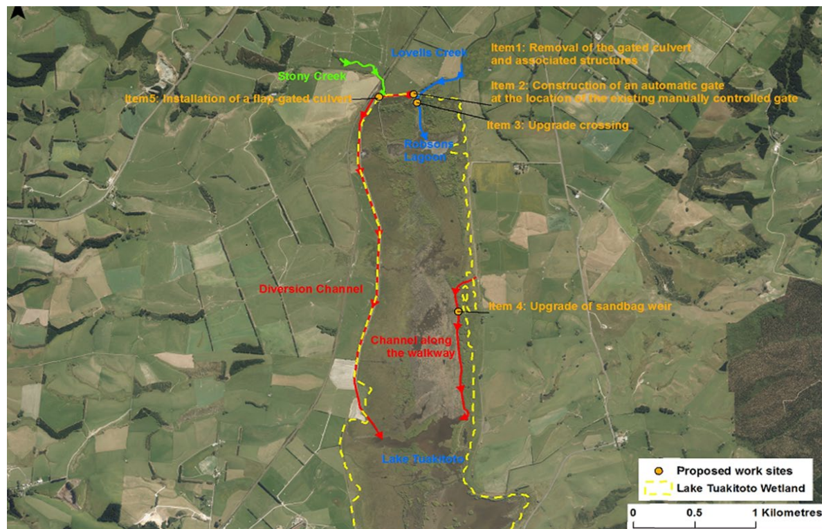
Figure 2. Plan of proposed flow structures upgrades.
