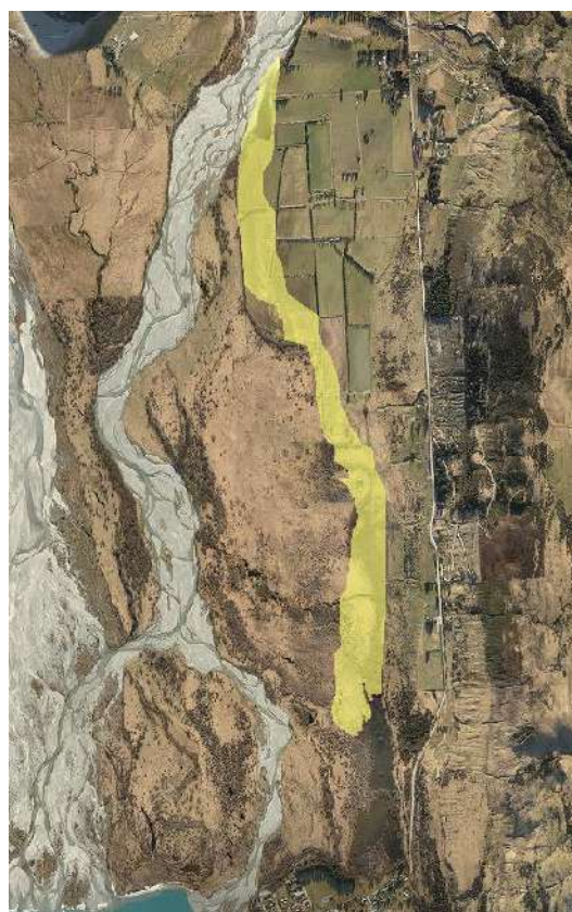
Figure 2.12: Possible channel avulsion path along left bank of Lower Rees River towards Glenorchy Lagoon
