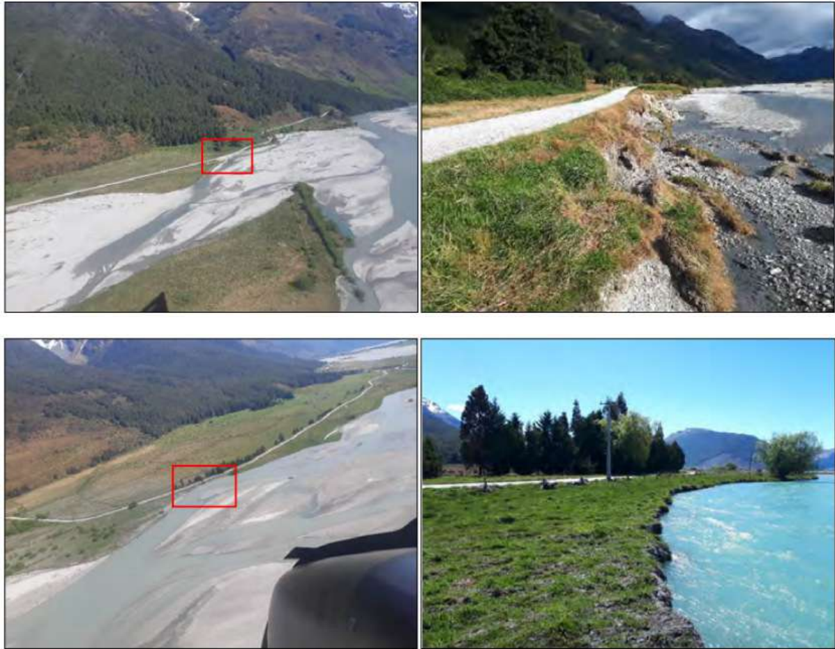
Figure 12: Aerial views (October 2020) of the Dart floodplain between Turner Creek and Kowhai Creek confluences (upper left) and between Glacier Burn and the Dart delta (lower left). Right-hand images show detail of erosion at these locations, taken February 2020 (upper right) and November 2020 (lower right).
