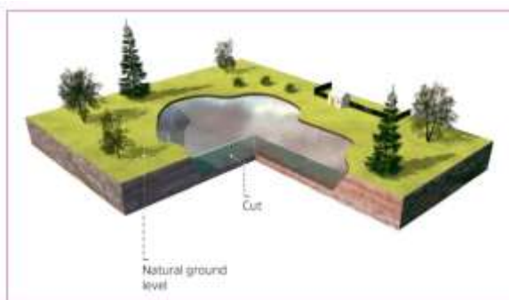
Figure 2 – pond cut into ground (no damming occurring)
