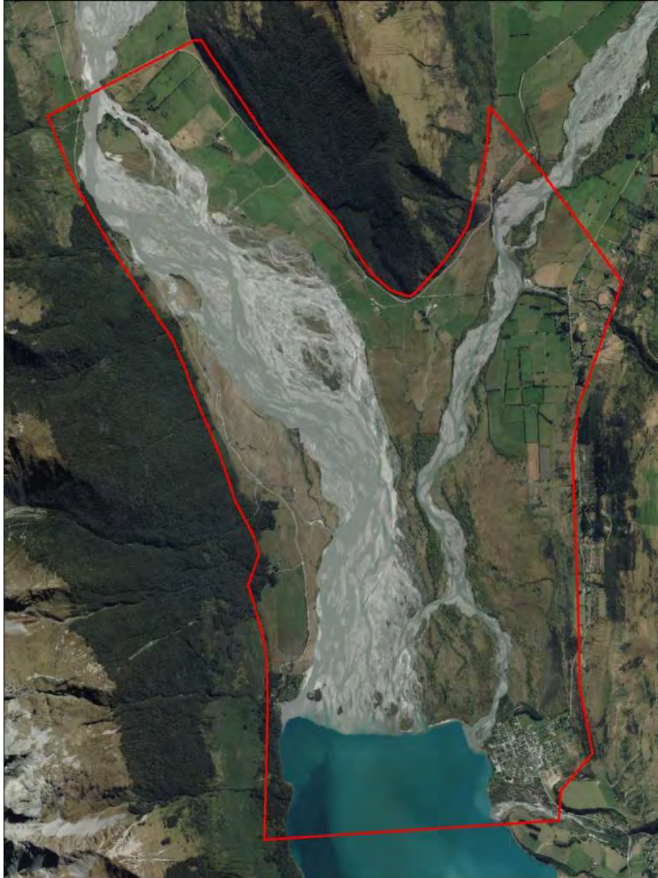
Figure 2.10: Extent of 2D computational hydraulic model of Dart-Rees River System used for flood hazard assessment
