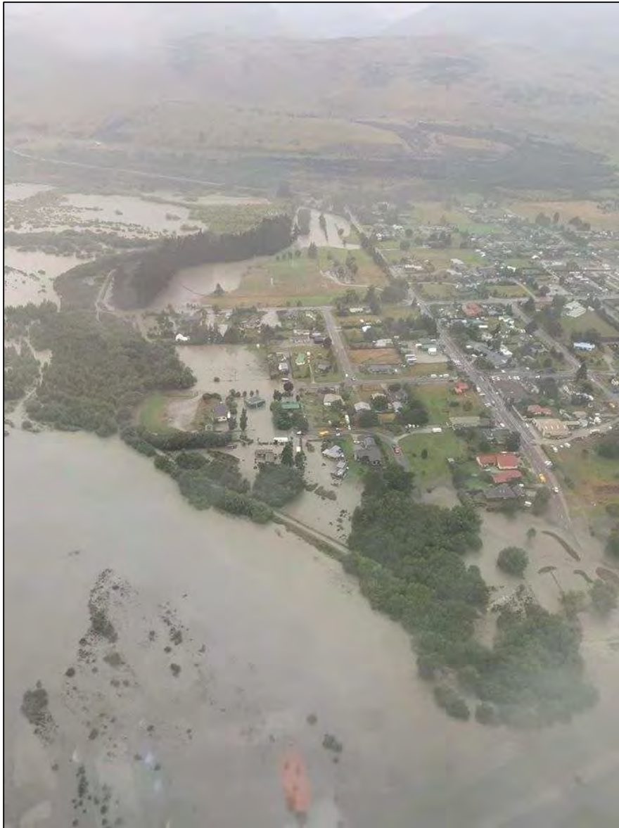
Figure 2: Flooding of the township in February 2020. In this event, floodwaters from the Rees River filled the Glenorchy Lagoon to the crest level of the adjacent Glenorchy floodbank and then overtopped to flow through the northwest margins of the township.
