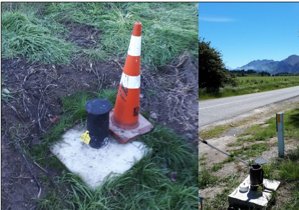
Figure 2: Examples of suitable, secure, purpose-drilled monitoring bores. Note the sealed concrete pad surrounding the bore head, raised casing above ground level, and the lockable cap.
