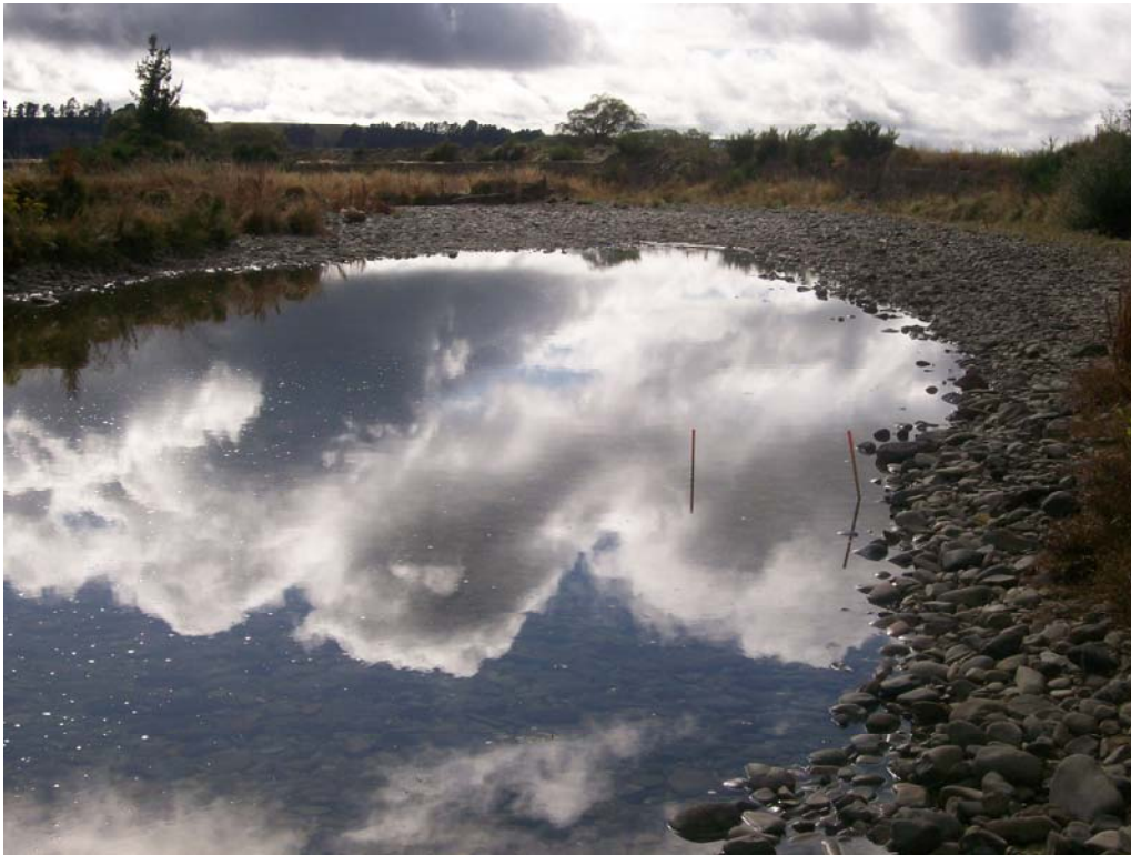
Figure 10: Kauru River gauging site (cross section 1) downstream view, 27 February 2007, flow approximately 0.03 \text{ m}^3/\text{s} .
