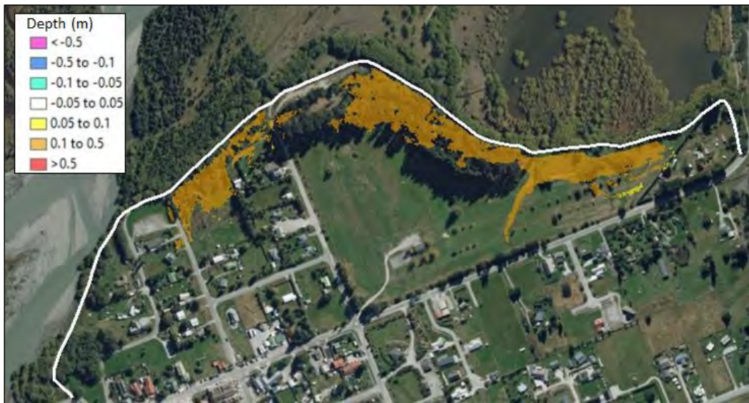
Figure 6-10 – Depth difference map between the 100m 3 /s aggradation (2m) and 300m 3 /s design (2019) runs. Despite the smaller flow, the aggradation scenario produces greater inundation.
