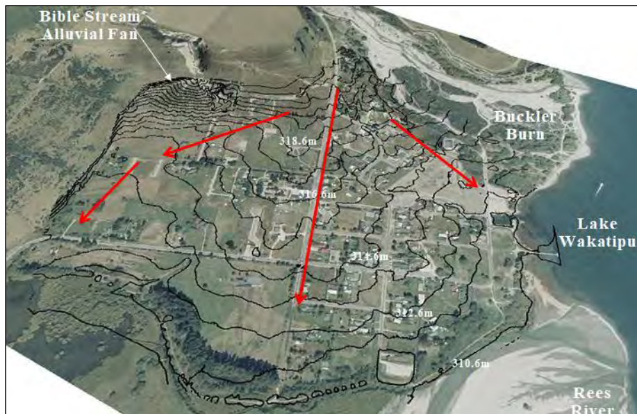
Figure 7-1 - ORC generated image. Land River Sea Buckler Burn model flow paths drawn on in red.
