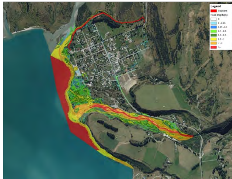
Figure 2: Model results for a Buckler Burn flooding scenario with a 300 cumec peak flow (<1% AEP). In this scenario minor floodwaters flow into the township area, mainly flowing northwards along Oban Street and around the eastern margin of the township. Colouring shows peak floodwater depths according to the included legend.
