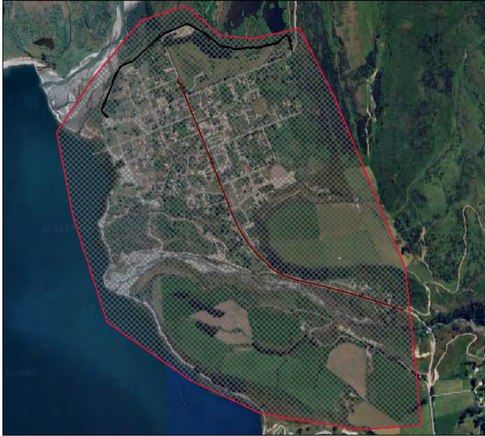
Figure 4-1 - Visualisation of the mesh with the inclusion of the Glenorchy stopbank (black line) and the Glenorchy-Queenstown Rd and Oban St break line (dark red).
