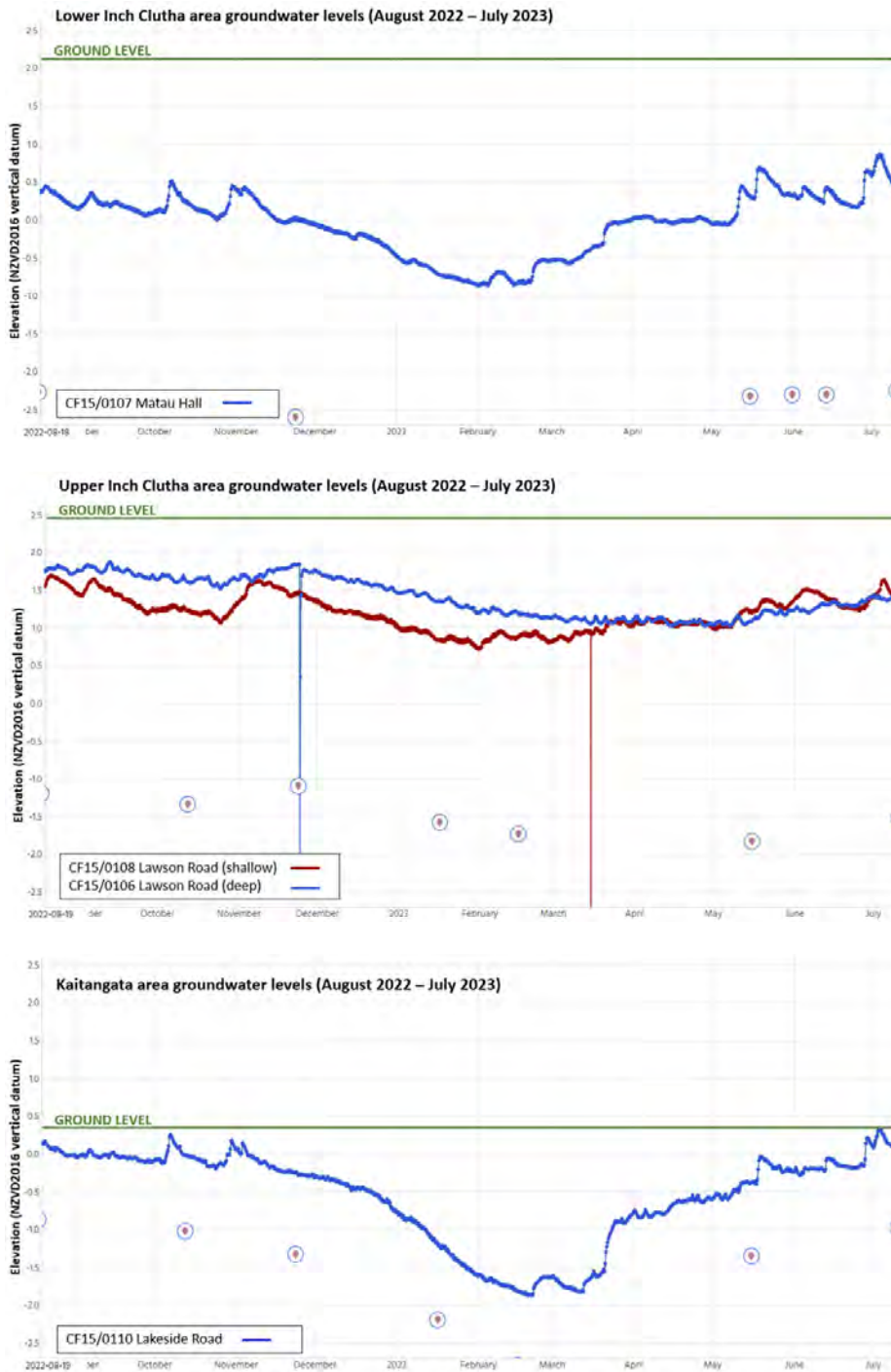
Figure 14: Groundwater level data from the lower Clutha Delta at Paretai, Inch Clutha and Kaitangata (August 2022 to July 2023), all levels are relative to NZVD2016 vertical datum. Bore locations are shown in Figure 12. These bores are all located within pumped drainage areas, so groundwater levels are lower than they would be if drainage was through gravitational processes only. Sharp downward dips in some plots are due to the taking of water samples in wells with a low yield.
