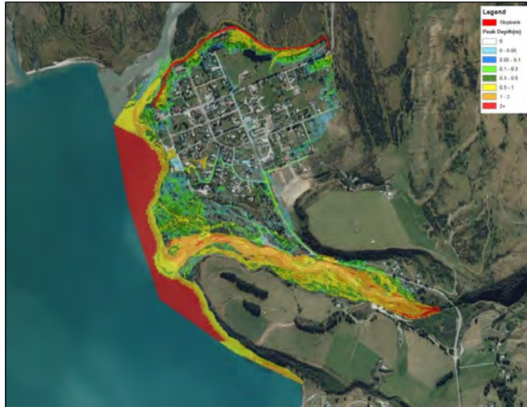
Figure 3: Model results for a Buckler Burn flooding scenario with a 300 cumec peak flow (<1% AEP) and a 3 metre thickness of channel aggradation on the mid-upper reaches of the alluvial fan. In this scenario floodwaters flow into the township area mainly flowing northwards along Oban Street, and along Invincible Drive and Shiel Street. Colouring shows peak floodwater depths according to the included legend. The flood hazard categorisation for this scenario is shown as Figure 4.
