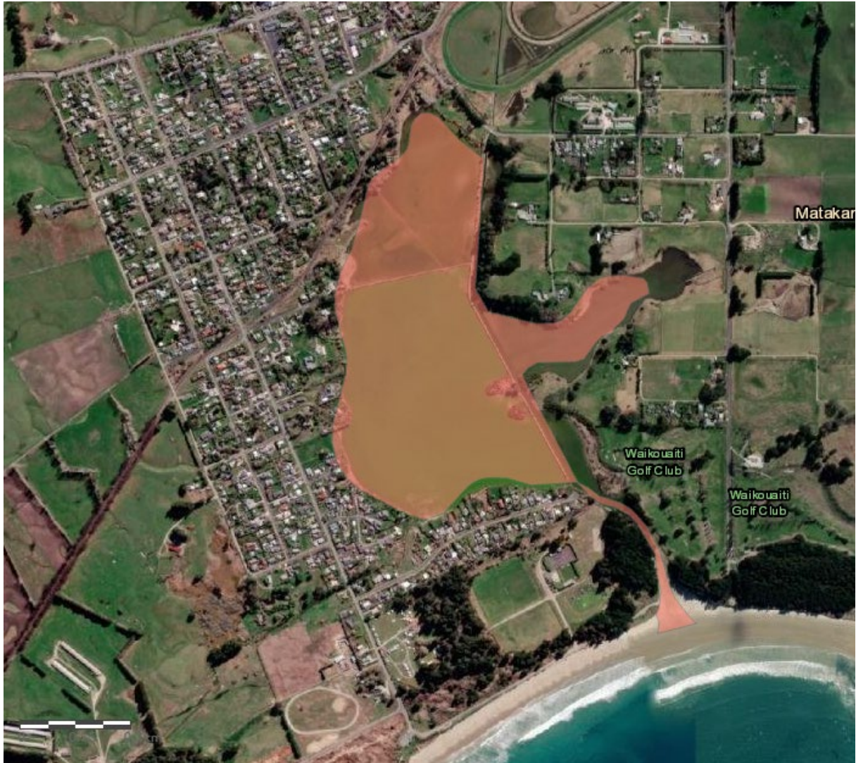
Figure A-6: Waikoaiti (Hawkesbury) Lagoon. Hawkesbury Lagoon is classified as a Beach Stream (damp sand plain lake) or coastal lake. The lagoon is segmented by causeways that will strongly influence circulation patterns and flushing, and the effect of these cannot be incorporated in single compartment models.
