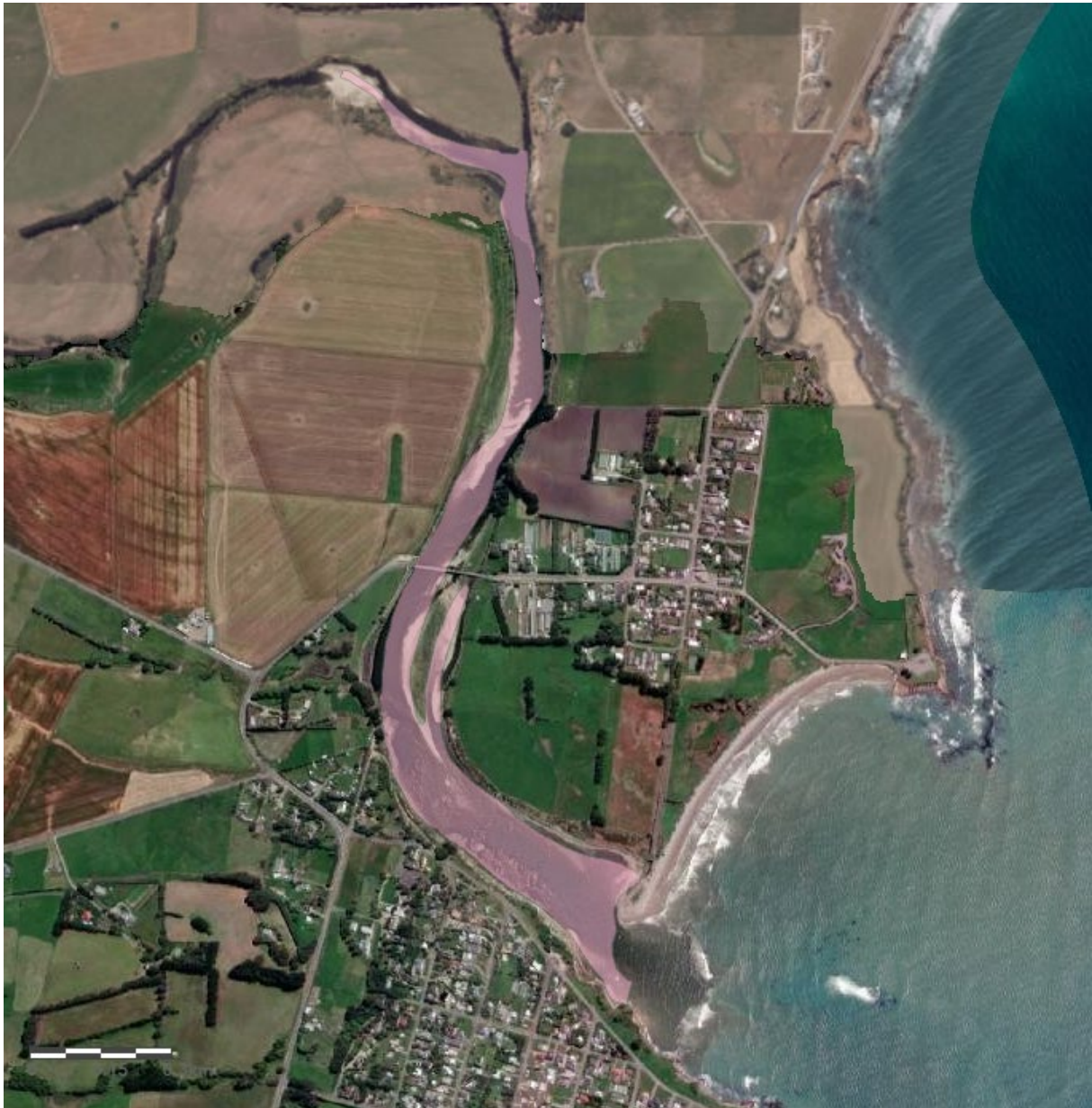
Figure A-1: Kakanui Estuary. The Kakanui Estuary is classified as a Tidal River Mouth (spit enclosed). It is also an ICOE, closing during periods of low flow. Tidal prism, volume, and area have been calculated from a bathymetry survey conducted by NIWA in 2015. The estuary extents shown are from Coastal Explorer and are consistent with the 2015 survey.
