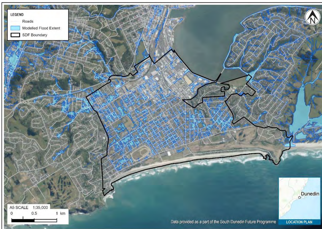
Figure 2.9 1% AEP current day flood model results of South Dunedin (Source: 2011 Integrated Catchment Management Plan 22 ).
