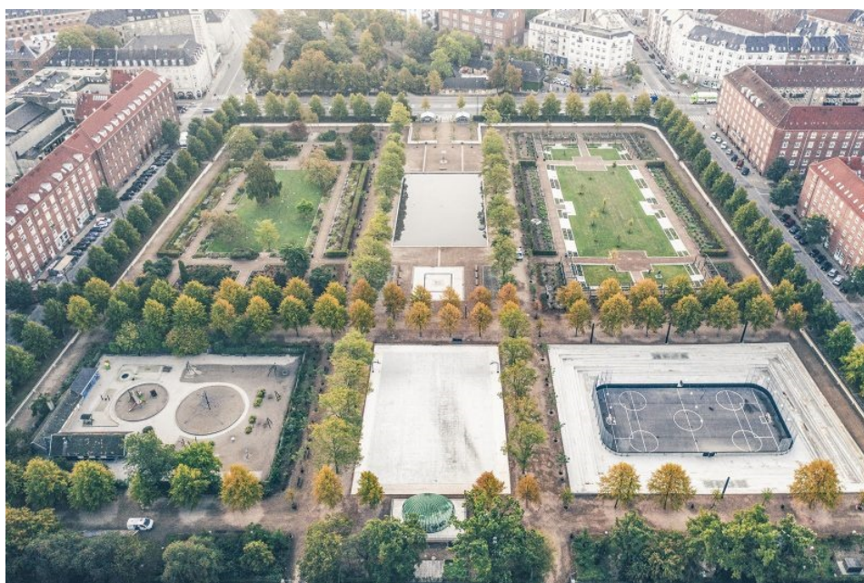
Figure 3.1: Enghaveparken in Copenhagen was transformed to hold up to 22,600 m 3 of rainwater [6].
