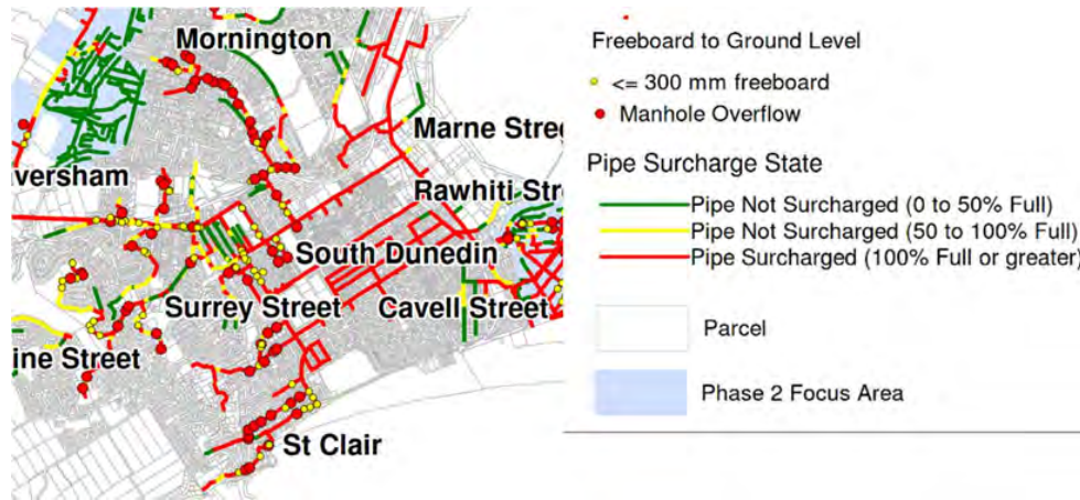
Figure 3.2 Snapshot of wastewater network surcharging and overflows, showing widespread surcharging and overflows of the wastewater network (Source: Dunedin ISP Programme).
