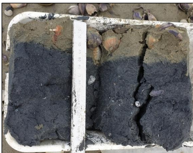
Example of distinct aRPD colour change with brown oxygenated sediments from the surface down to ~40mm
