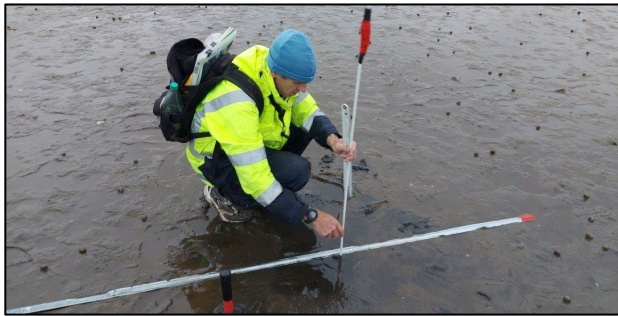
Installing sediment plates at Site A (top) and measuring sediment plate depths (bottom)
