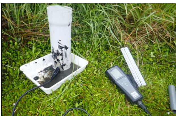
Oxidation reduction potential measurement with probe inserted horizontally into core. Where in situ measurement is not possible, cores are extracted and placed on a tray.
