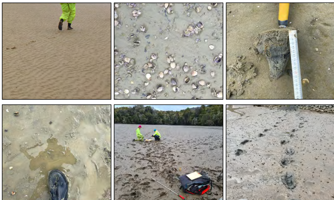
Examples of substrate types: Top row (L to R); mobile sand (0-10%), firm shell/sand (0-10%), firm sand (0-10%), Bottom row (L to R); firm muddy sand (10-25%), soft muddy sand (25-50%), very soft sandy mud (50-90%).
