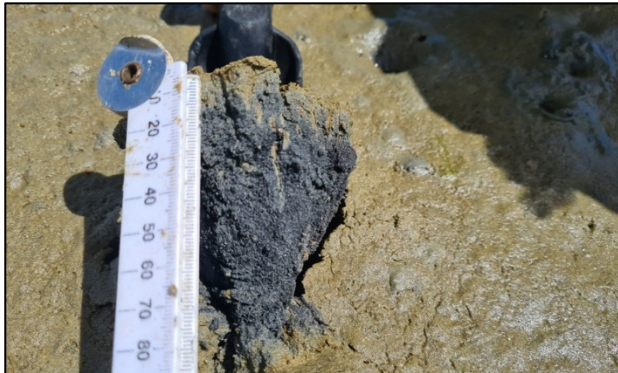
Example of distinct colour change with depth, showing brown oxygenated sediments on the surface down to ~10mm
