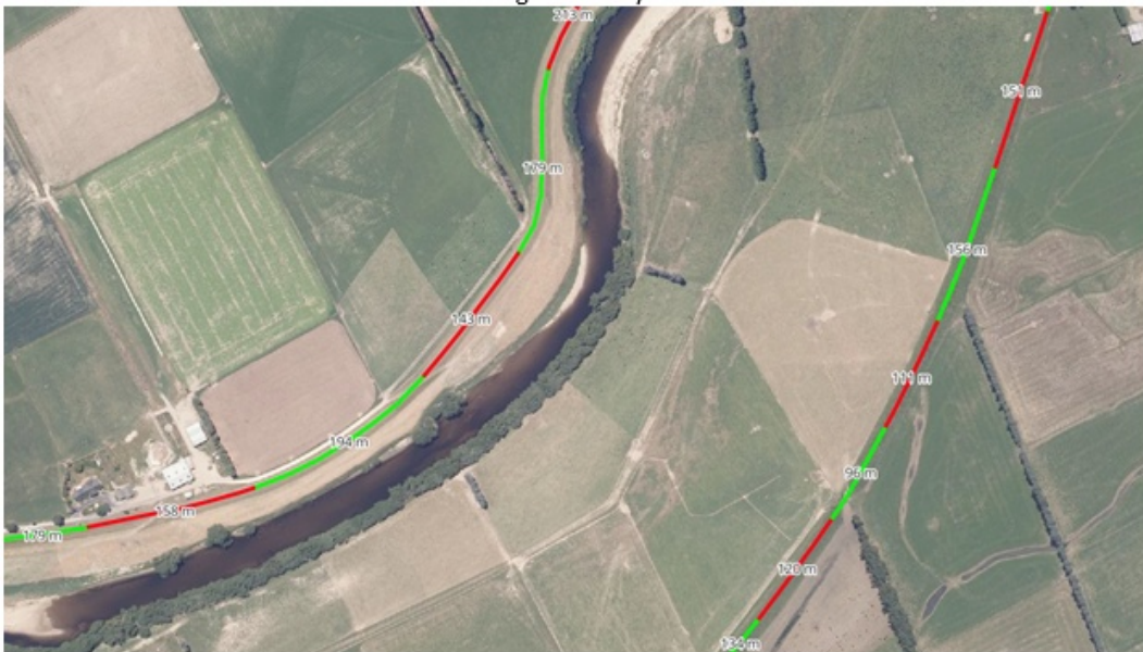
Figure 11: A zoomed-in section of part of the Taieri River as an example of the delineation of floodbanks (the colours distinguish each segment and do not represent asset condition or failure risk and the numbers demonstrate section length in metres).
