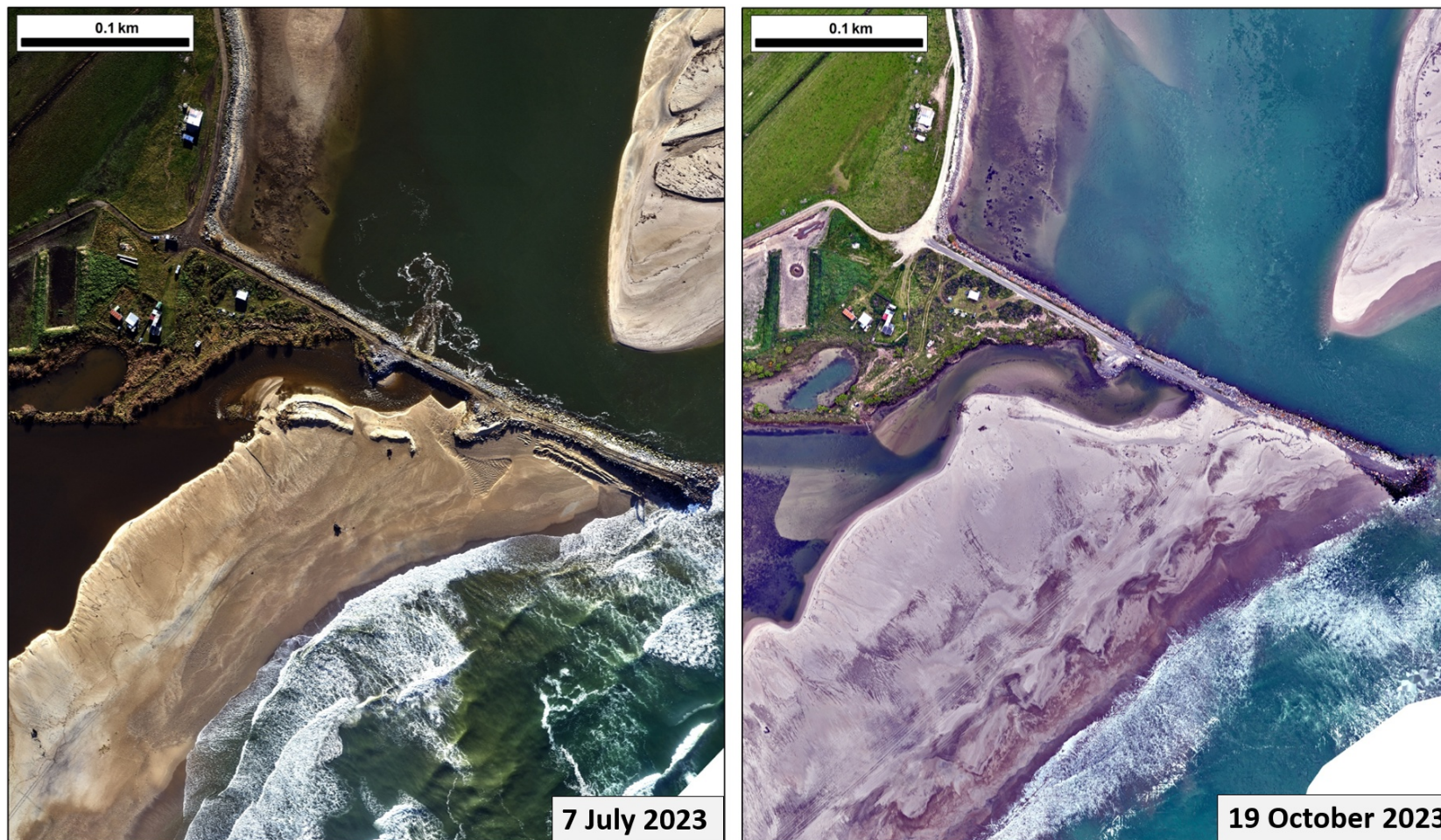
Figure 7: Aerial imagery showing a closer view of the Koau Mouth training line and Puerua estuary in July and October 2023.
