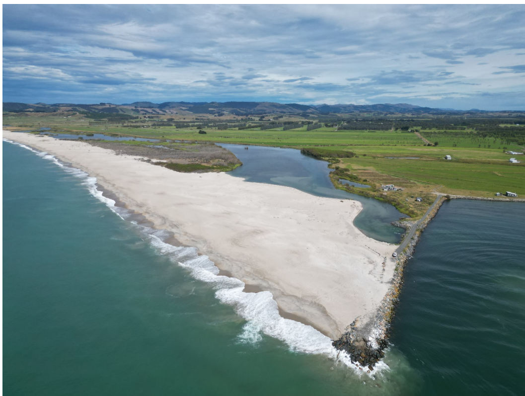
Figure 9: Imagery showing the Koau training line (holds culverts) and the progression of the sand deposition, 19 January 2024.
