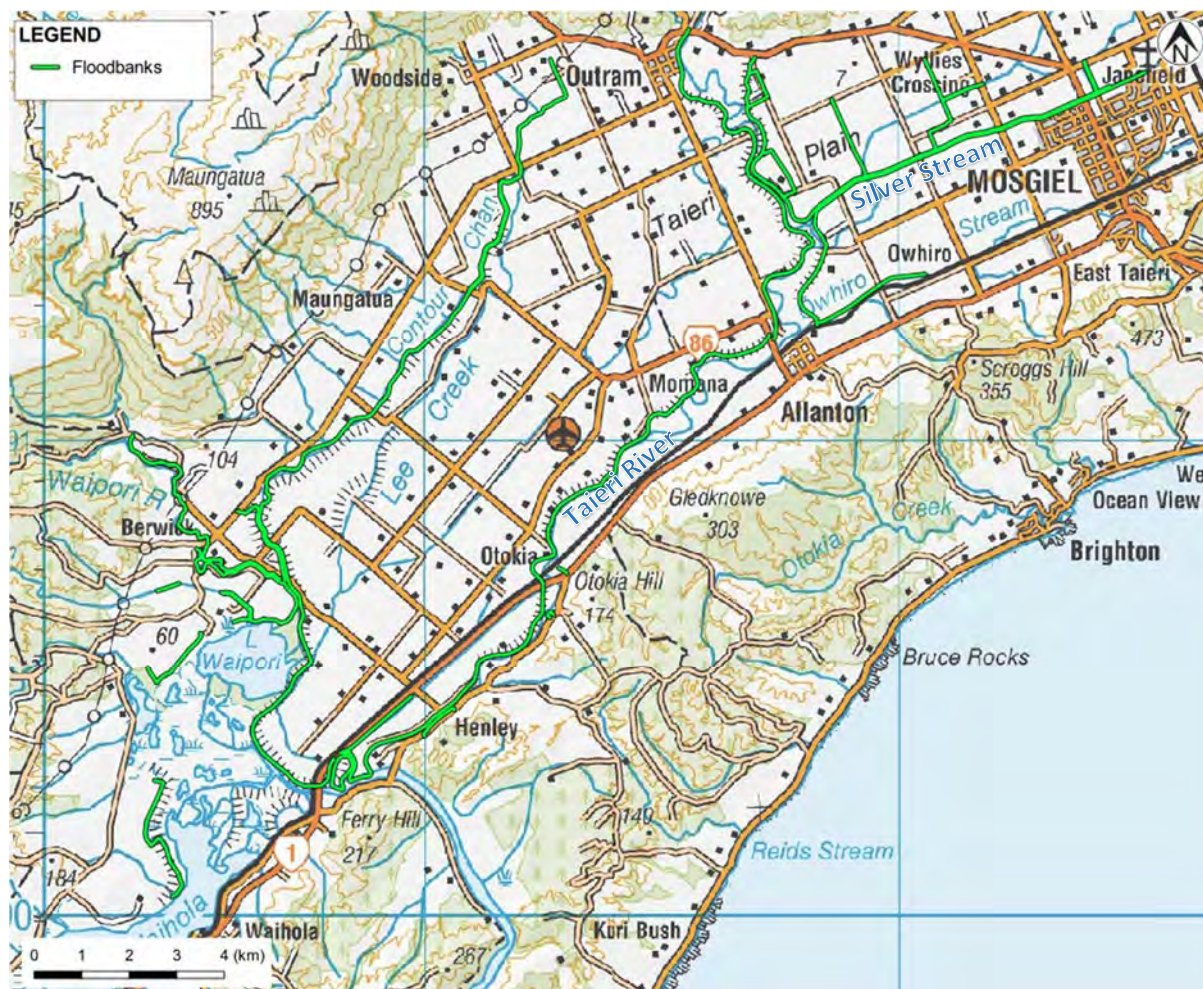
Figure 3: Lower Taieri River Flood Protection Scheme assessed floodbanks
