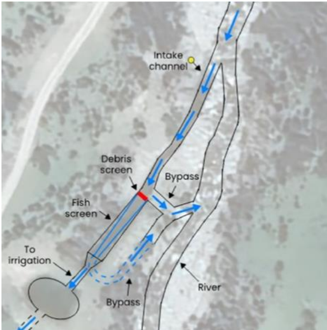
Figure 1: Schematic diagram of a likely water take scenario across the Otago region.
