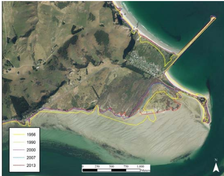
Figure 41 Changes in the Aramoana coastline between 1956 and 2013, overlaid on an aerial photograph collected in 2013 (source: DCC)
