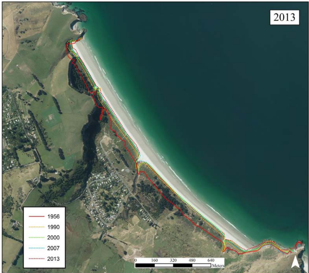
Figure 47 Changes in the location of the vegetated foredune at Long Beach between 1956 and 2013, overlaid on an aerial photograph collected in 2013 (source: DCC)
