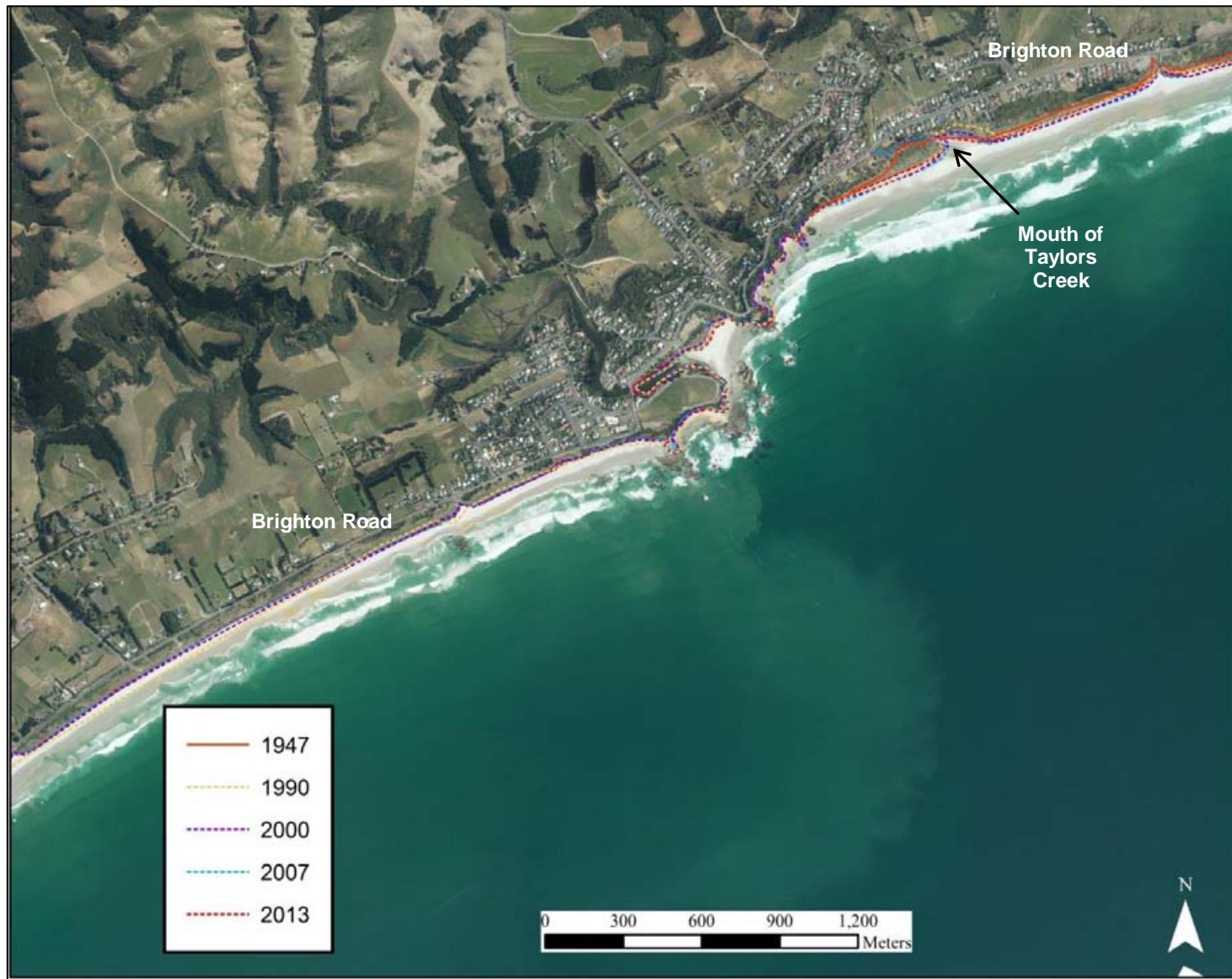
Figure 7 Changes in the Brighton coastline between 1947 and 2013, overlaid on an aerial photograph collected in 2013 (source: DCC)
