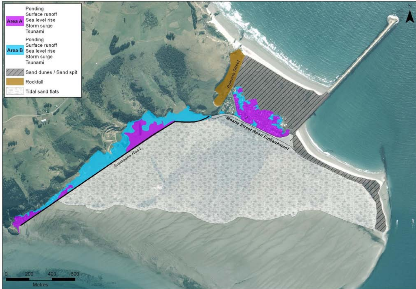
Figure 38 Mapped natural hazard areas in the Aramoana / Te Ngaru area
