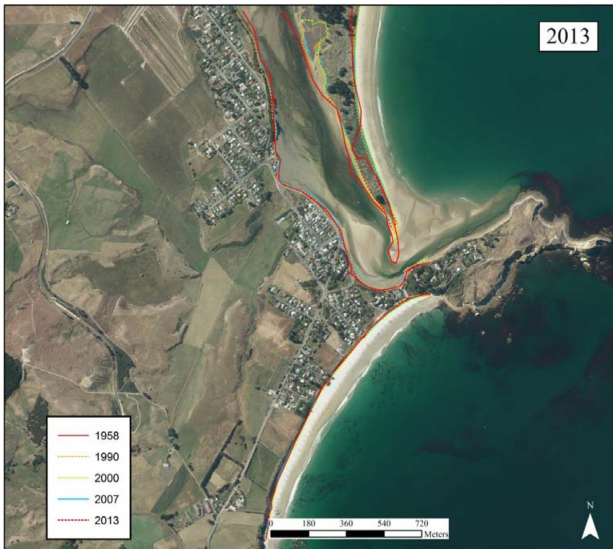
Figure 65 Changes in the Karitane coastline between 1958 and 2013, overlaid on an aerial photograph collected in 2013 (source: DCC)
