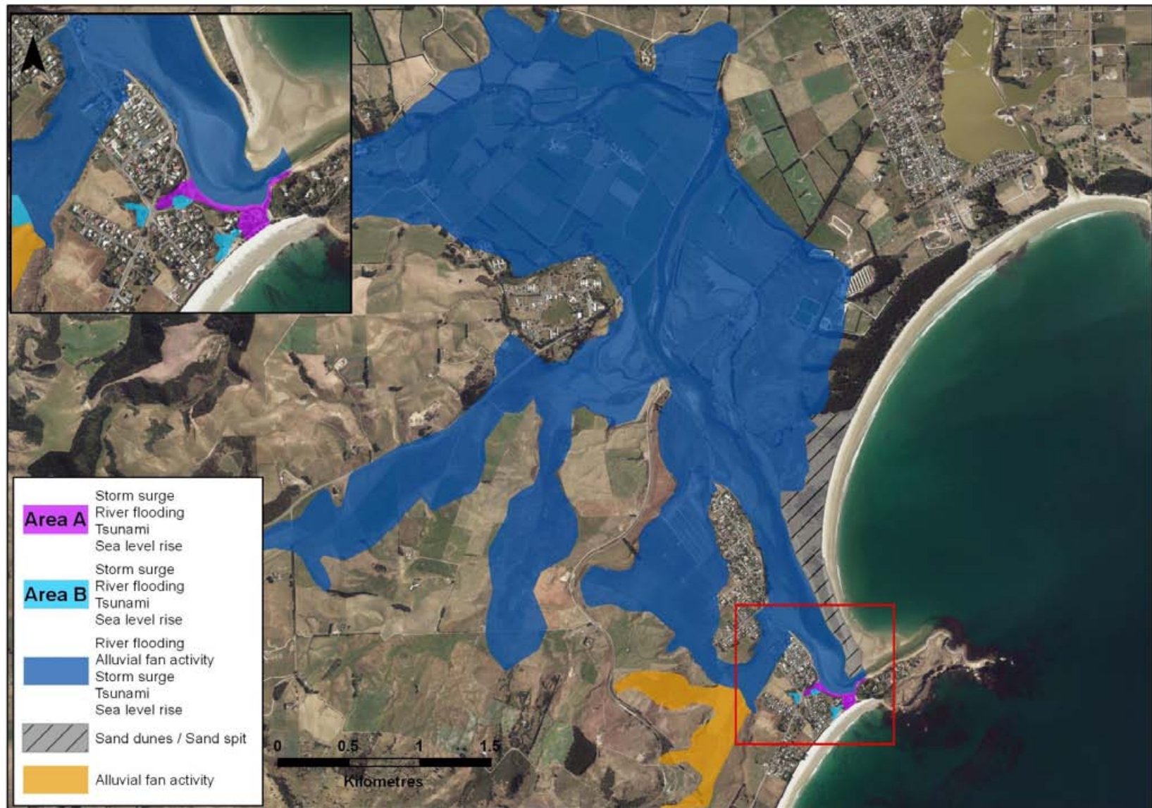
Figure 63 Mapped natural hazard areas in the vicinity of Karitane, and at the mouth of the Waikouaiti River (inset)
