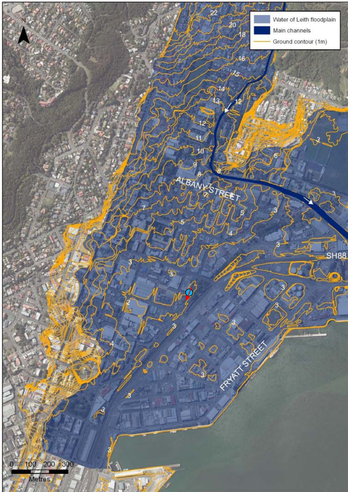
Figure 32 Water of Leith - CBD reach floodplain area. The approximate direction and location of the photo in Figure 10 is also shown. The topography of the area to the south of Jetty Street is shown in Appendix 5.
