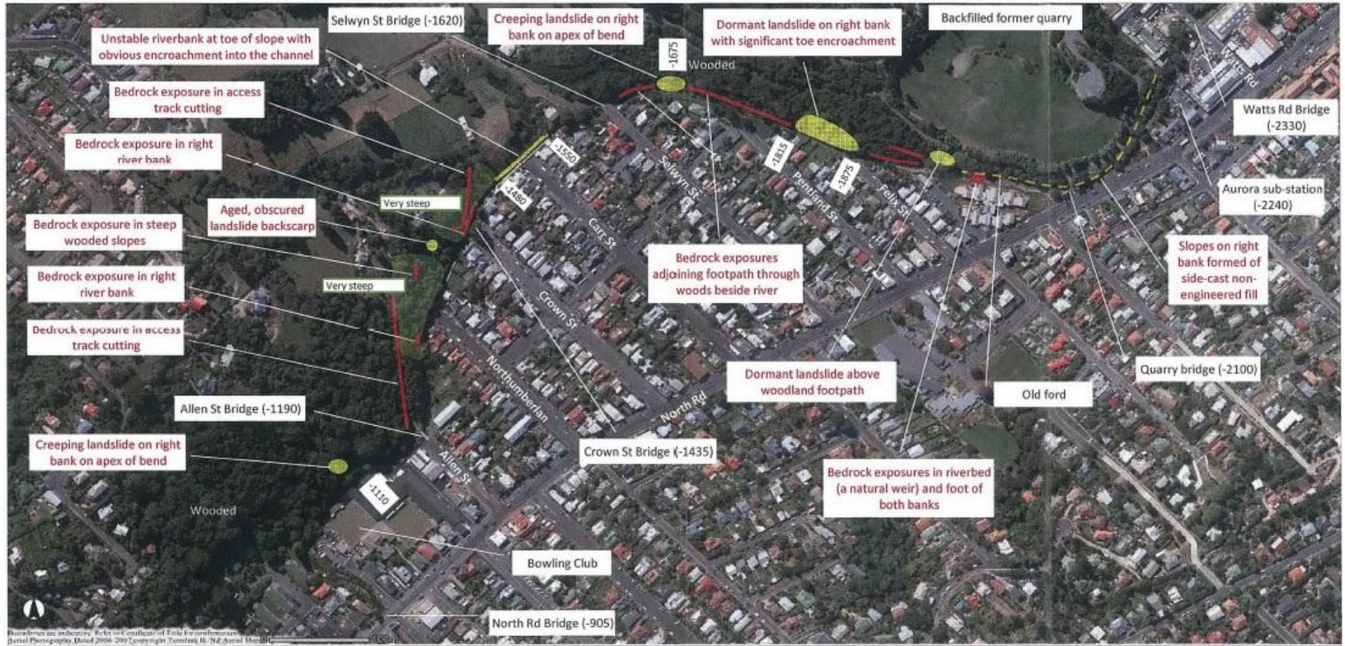
Figure 21 Geological summary map of Lindsay Creek between Watts Road and North Road bridge, as prepared by Coffey (2010)
