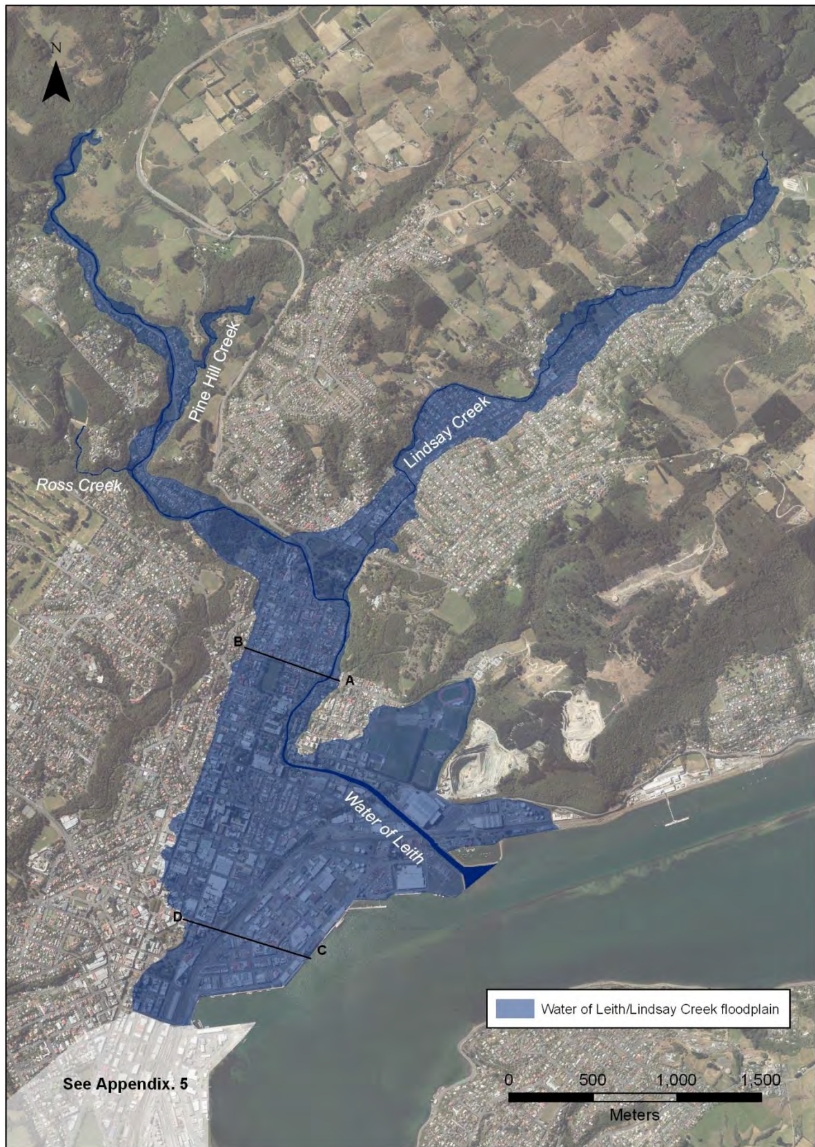
Figure 12 Water of Leith and Lindsay Creek mapped floodplain area. The location of the cross sections shown in Figure 13 and Figure 14 is also shown. The topography of the area to the south of Jetty Street (shaded white) is shown in Appendix 5.
