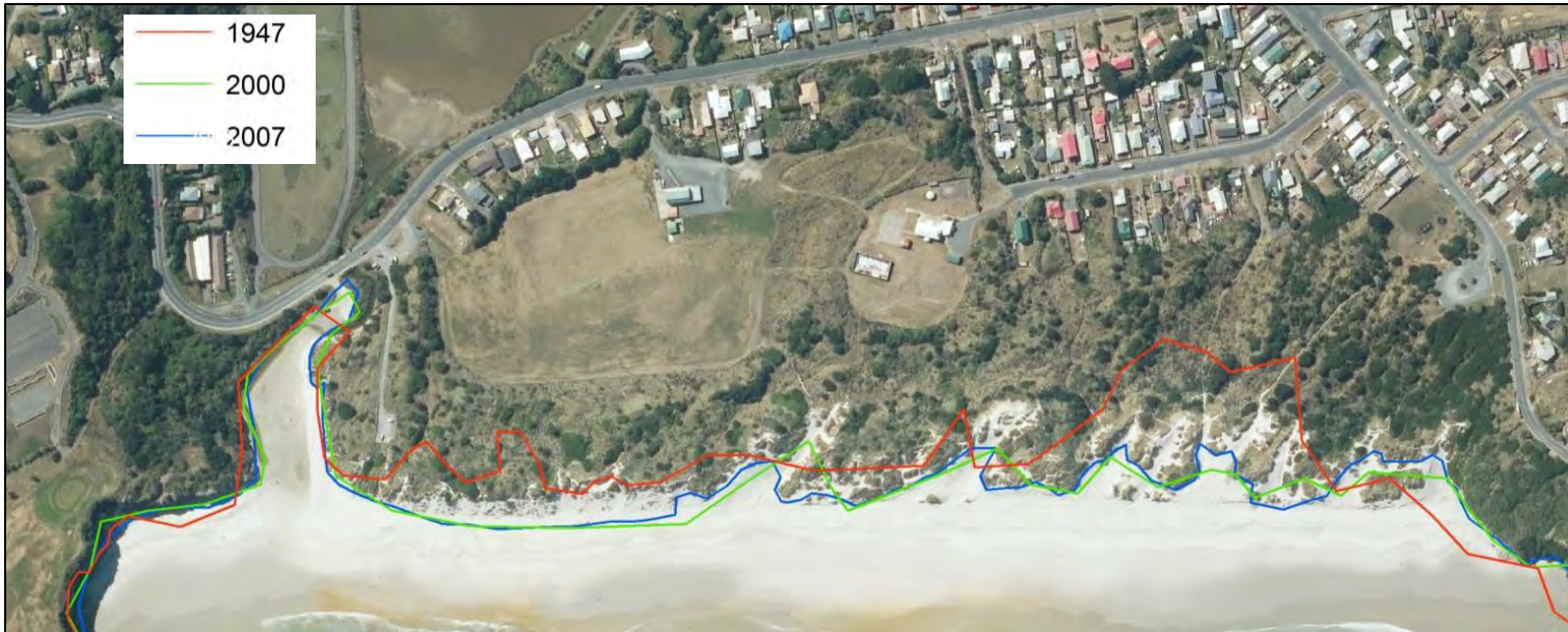
Figure 22. Changes in the Ocean Grove coastline between 1947 and 2007, overlaid on an aerial photograph collected in 2013 (Source: DCC)
