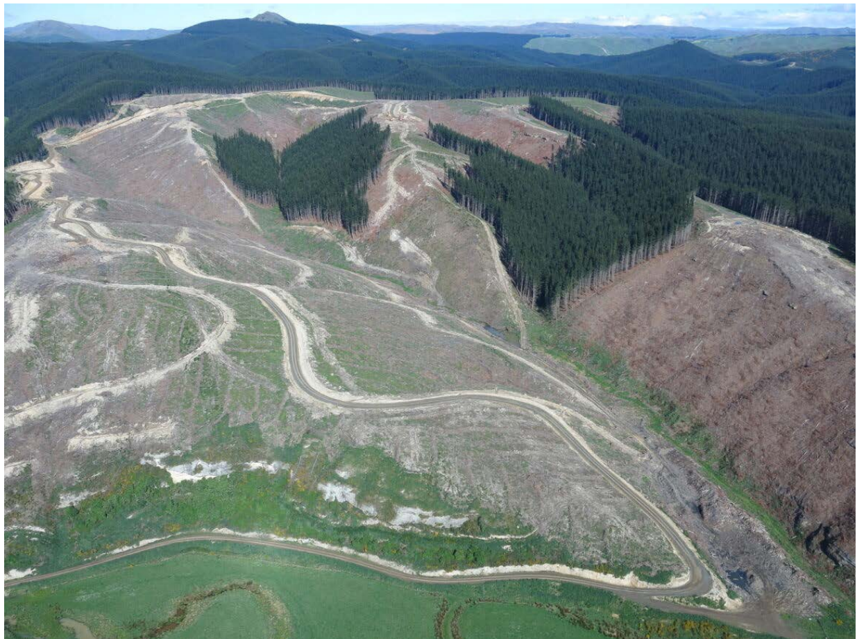
Image 10: Post discharge event (approx. 18 months) – Gradient of road from aerial footage. Point of discharge was located at the bottom right road bend of image
