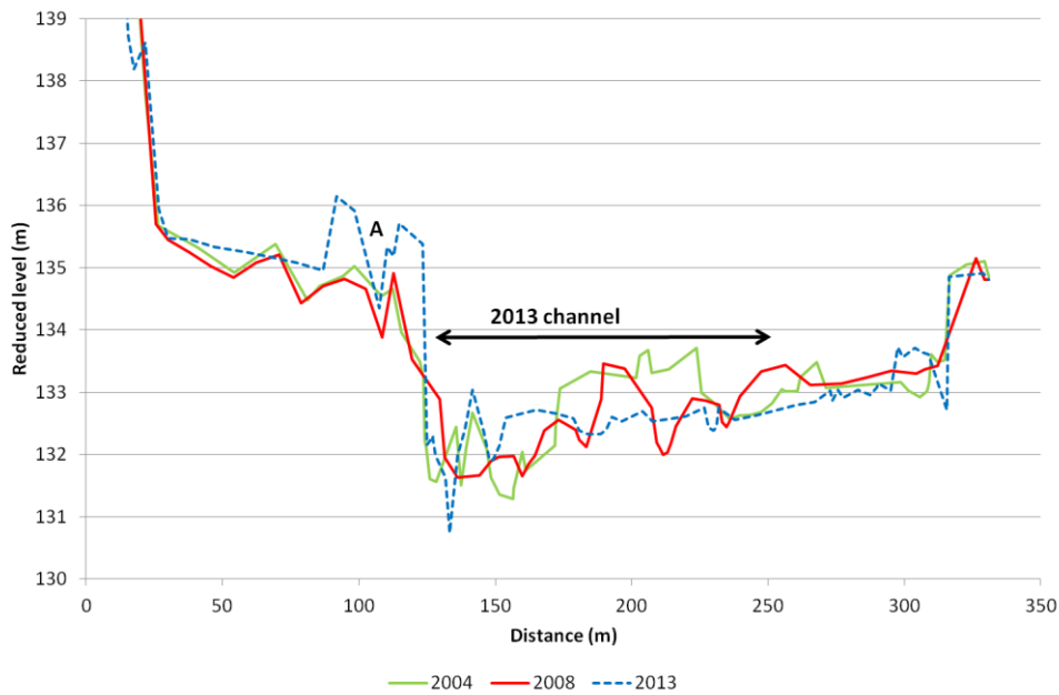
Figure 29- Cross-section WA5N, looking downstream
