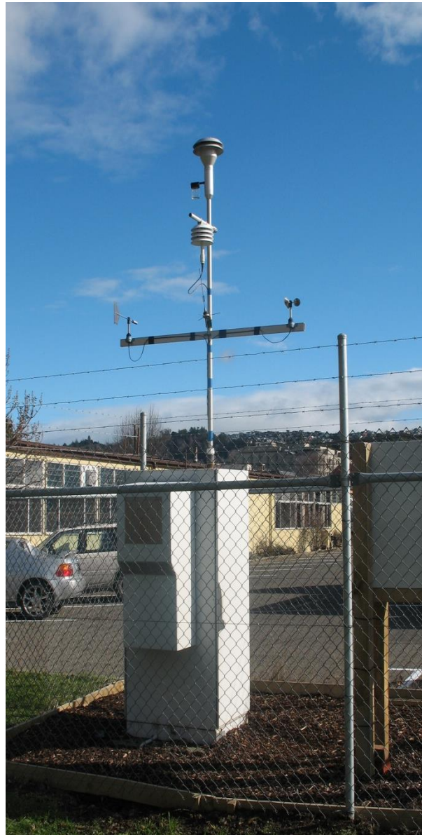
Figure 2. A typical BAM1020 installation. The station at Dunedin measures PM_{10} , air temperature, wind speed and direction. The PM_{10} sampling inlet is shown at the top.
