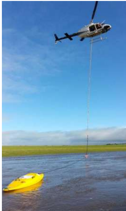
Figure 53. Heli-gauging underway on the Tokomairiro River using a kayak-mounted Acoustic Doppler Current Profiler (ADCP) flow measuring device
