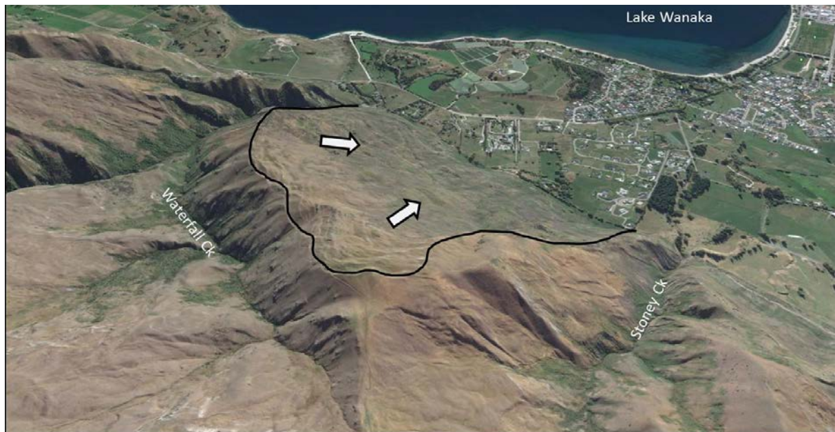
Figure 28. Oblique view towards the north, with downtown Wanaka visible in top right of image. A large deep-seated schist landslide south of Wanaka is outlined in black. Ridgeline relaxation can be seen at the top of the landslide.
