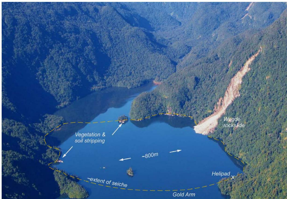
Figure 9. The 2003 Fiordland earthquake caused a 200,000 m 3 rockslide into Charles Sound. The landslide caused a small tsunami which ran 4-5 m up the other side of the sound, approximately 800 m away. (Hancox et al., 2003).
