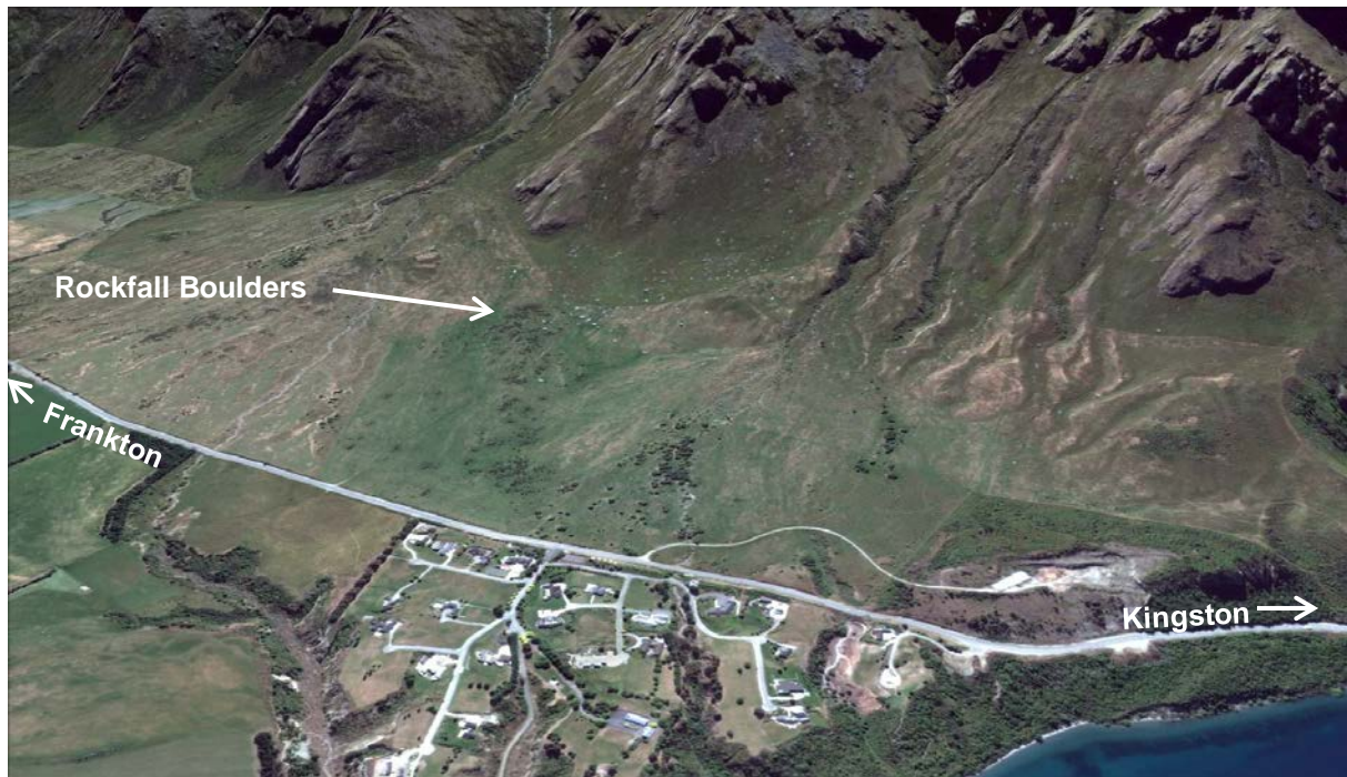
Figure 42. Oblique view towards the foothills of the southern Remarkables Range. SH6 runs across the lower view, with Lake Wakatipu lower right. Large boulders, likely from a rockfall, can be seen on the slopes below the rocky cliffs in the middle of the view (white dots). Active alluvial fans drain the catchments (view from Google Earth).
