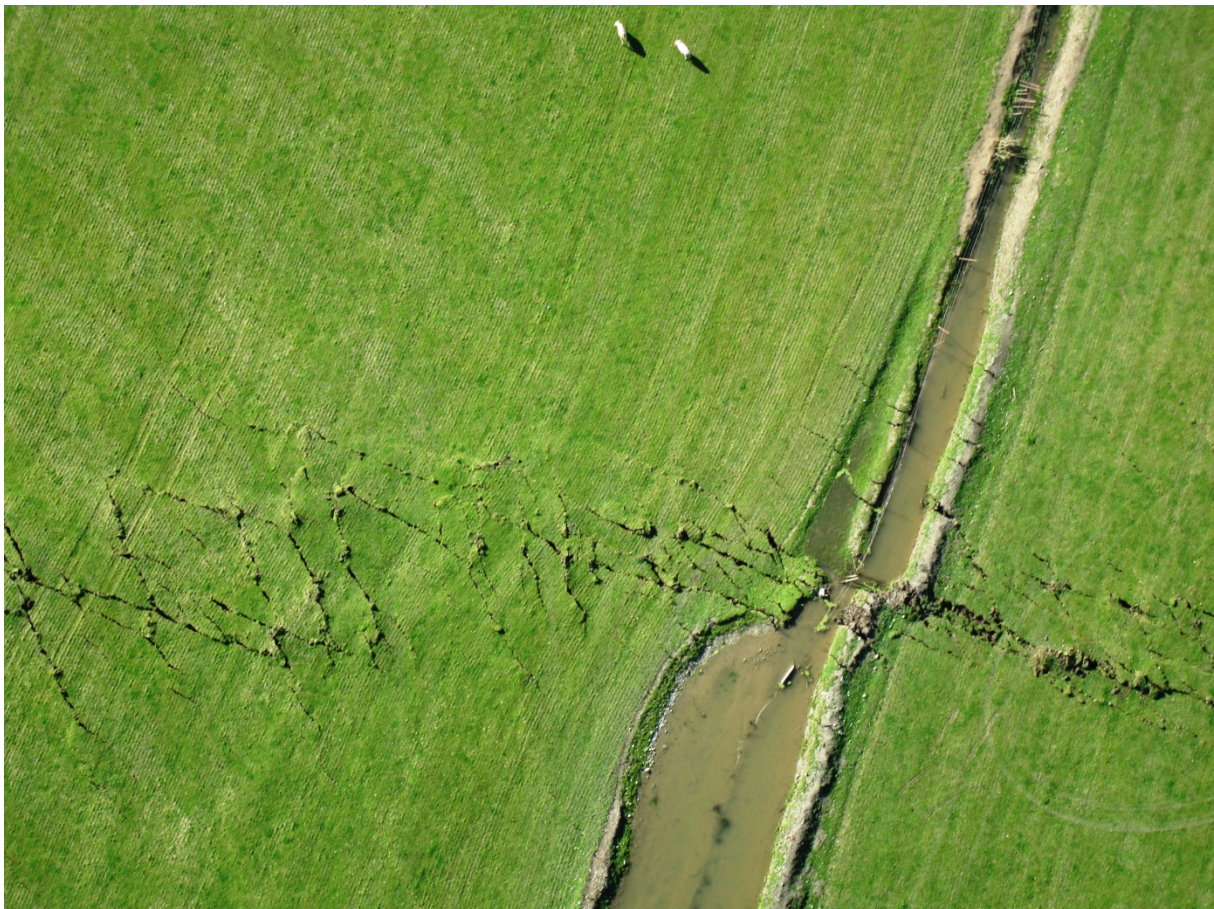
Figure 1. The surface trace of the Greendale Fault rupture cut across paddocks in the Canterbury Plains in September 2010. (Photo courtesy M. Quigley). The ground moved up to 5.3 m laterally, but was expressed at the surface as a zone of distributed deformation up to 300 m wide, seen in the network of shear structures (Quigley et al., 2012).
