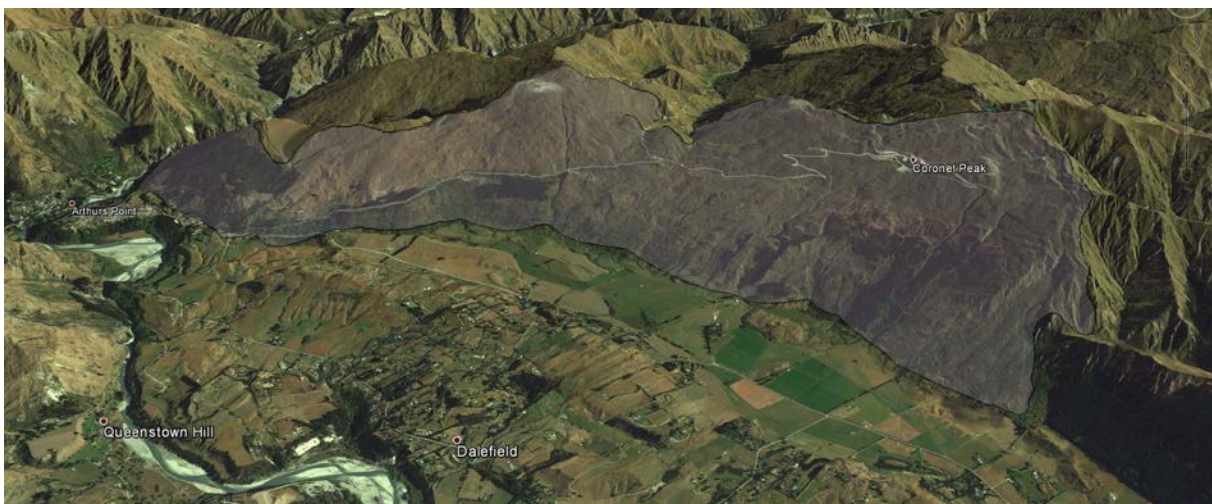
Figure 43. Oblique view showing outline of the Coronet Peak landslide, a large deep-seated schist landslide. The Shotover River runs along the left side of the image. (Google Earth).
