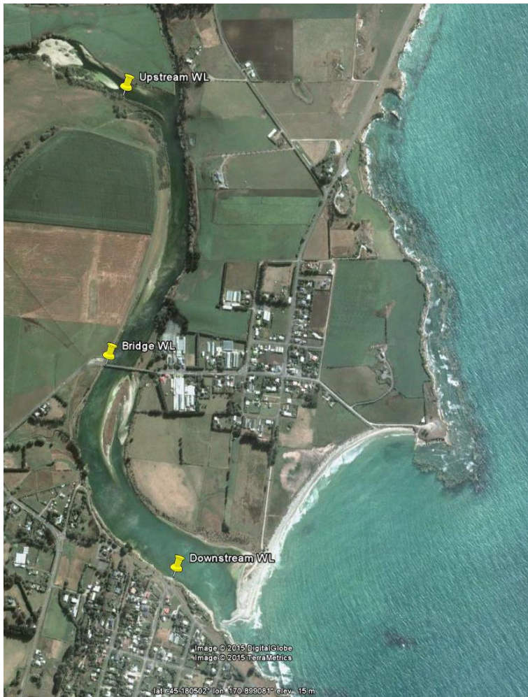
Figure 2-2: Location of water level recorders in the Kakanui Estuary.
