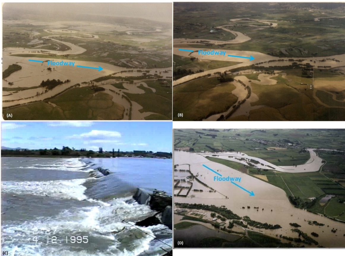
Figure 4.23 The Lower Clutha Floodway operating during October 1978 (a), January 1980 (b), December 1995 showing the floodway gates partially dropped (c) and November 1999 (d) flood events.
