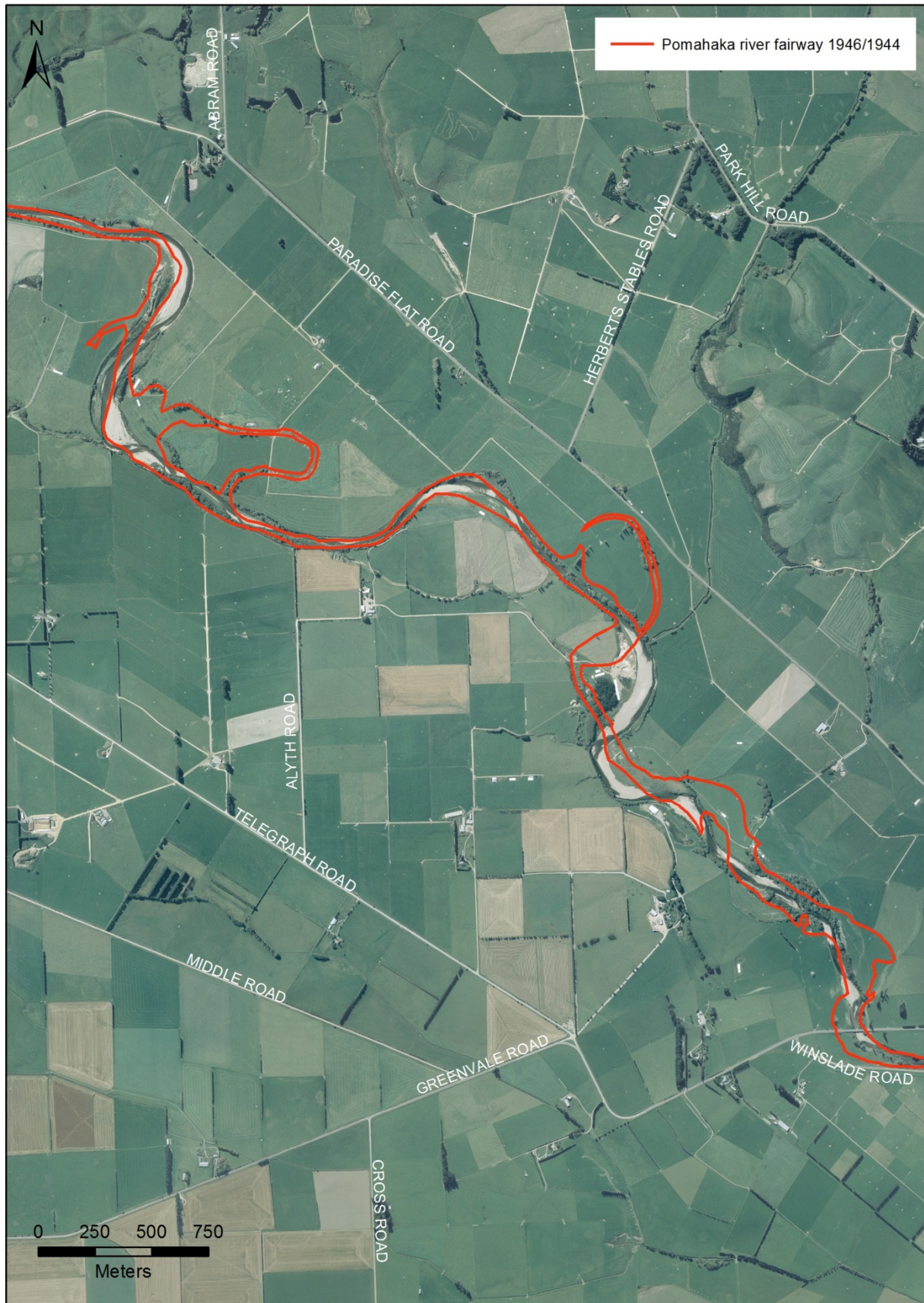
Figure 14. Comparison of the Pomahaka River between 1944/1946 and 2006 between Camperdown Bend and the Greenvale Road bridge (aerial photograph collected in 2006)
