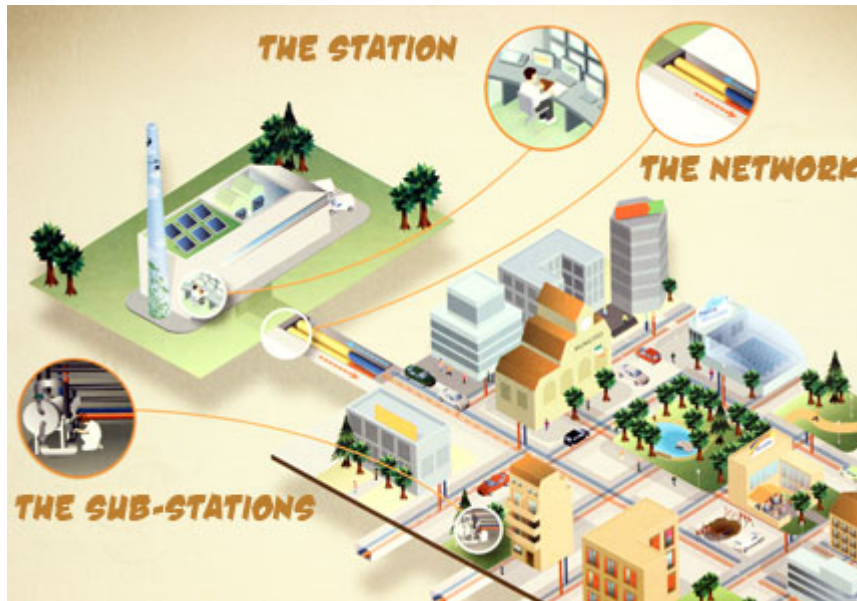
Figure 3. Schematic of a district-heating scheme.
