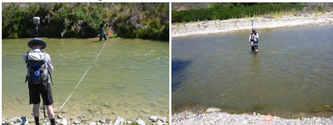
Figure 4: Hydraulic field data collection on the Manuherikia River. The hydraulic data underpins the IFIM model.
