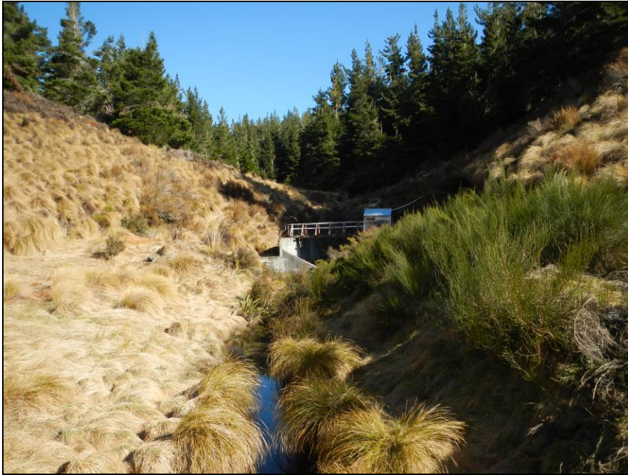
Figure 6. Photo of the flow and turbidity measuring station for the Forest catchment.
