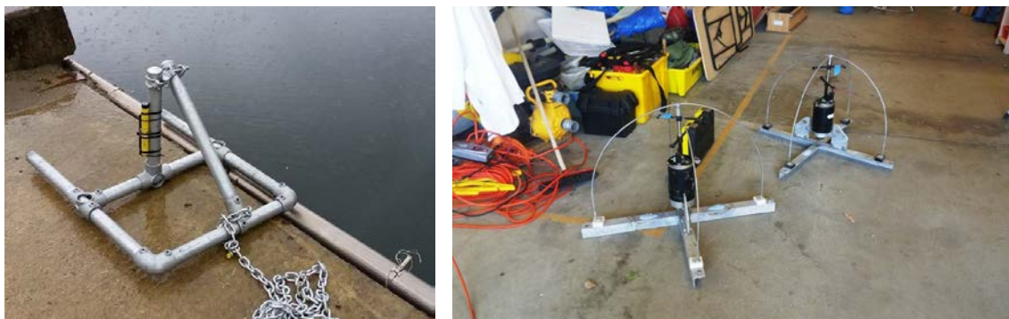
Figure 7: Conductivity/temperature sensor (left) and Acoustic Doppler Current Profilers (ADCP) (right) ready for deployment on the Waikouaiti River in support of Waikouaiti estuary model development.
