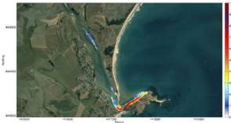
Figure 5 Example of modelling showing sediment mobilisation.
