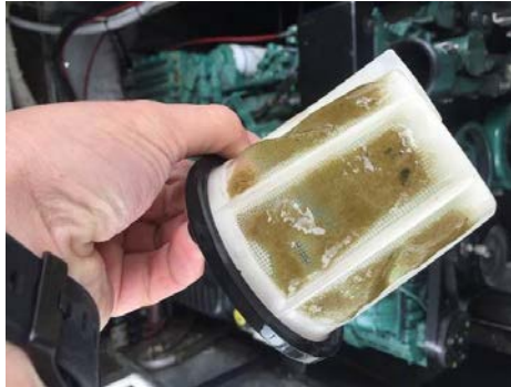
Figure 1. Photo of blocked boat engine water intake filter from Lake Wakatipu, May 2016.
