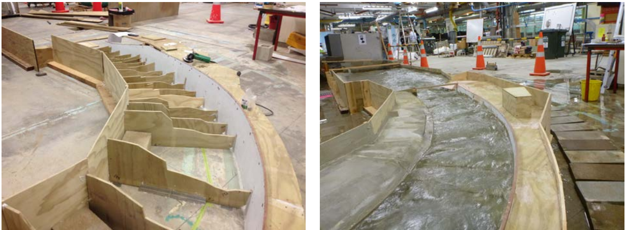
Figure 2: Progress on the construction of the physical hydraulic model for the Water of Leith between the Union Street Bridge and Clyde Street Bridge (left: model during the construction phase on 4 August 2016; right: model at the beginning of the calibration phase on 7 August 2016).
