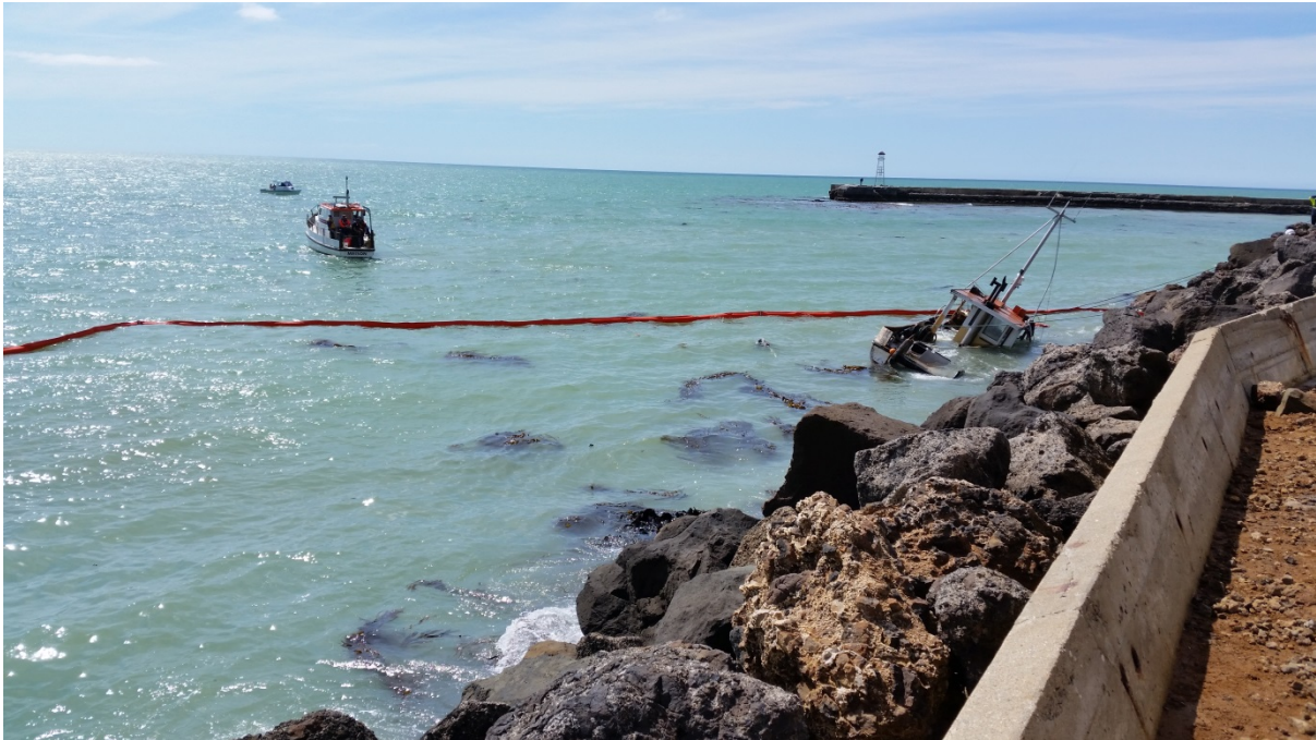
Rapid deployment boom secured around the Jane Marie
