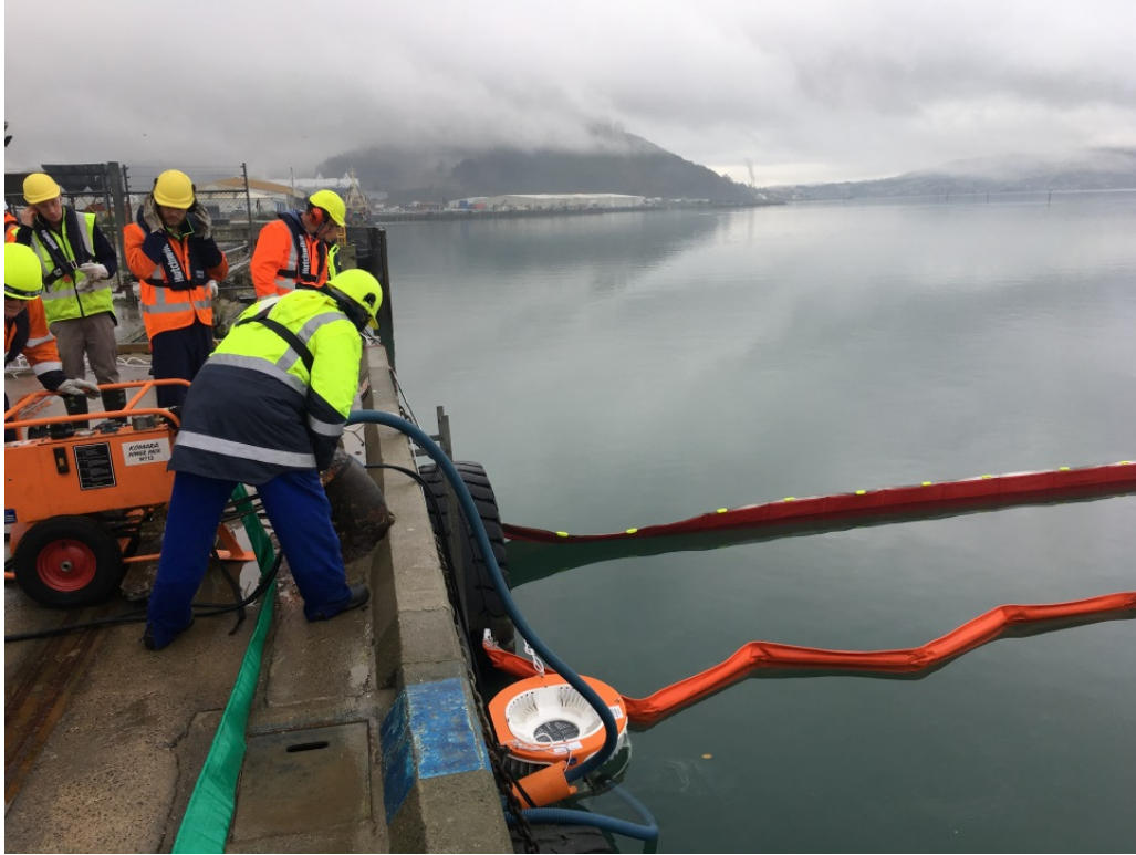
Staff deploy an oil “skimmer” during a marine oil spill training exercise on the Otago harbour.
