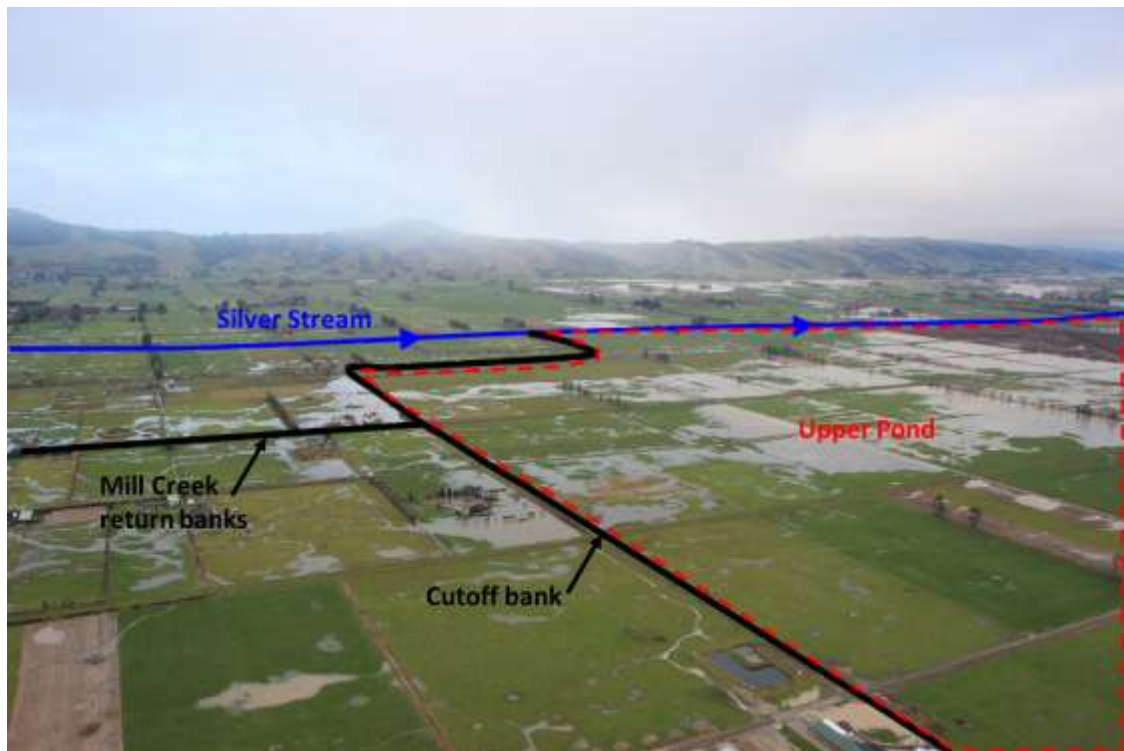
Figure 42. Ponding behind the Cutoff Bank; view is towards the south – 4 June 2015
