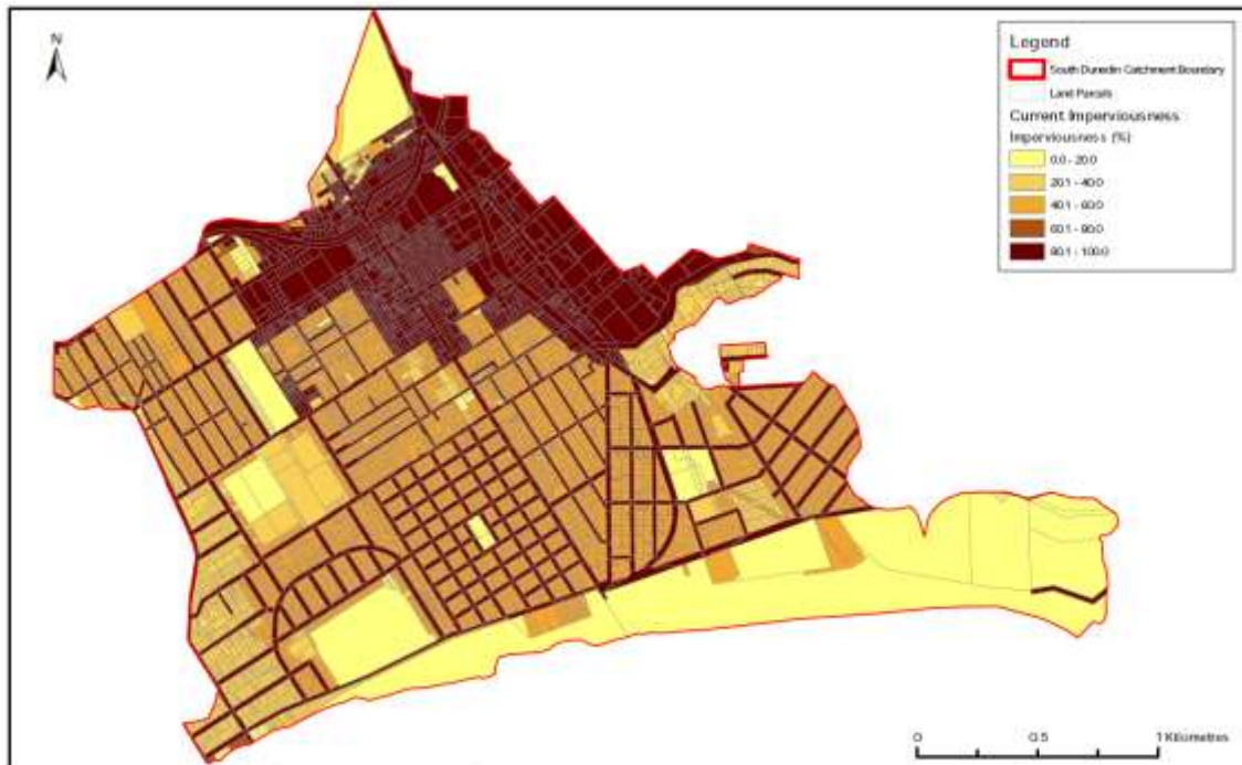
Figure 26. Map showing the current level of imperviousness, as defined by URS and Opus for the DCC
