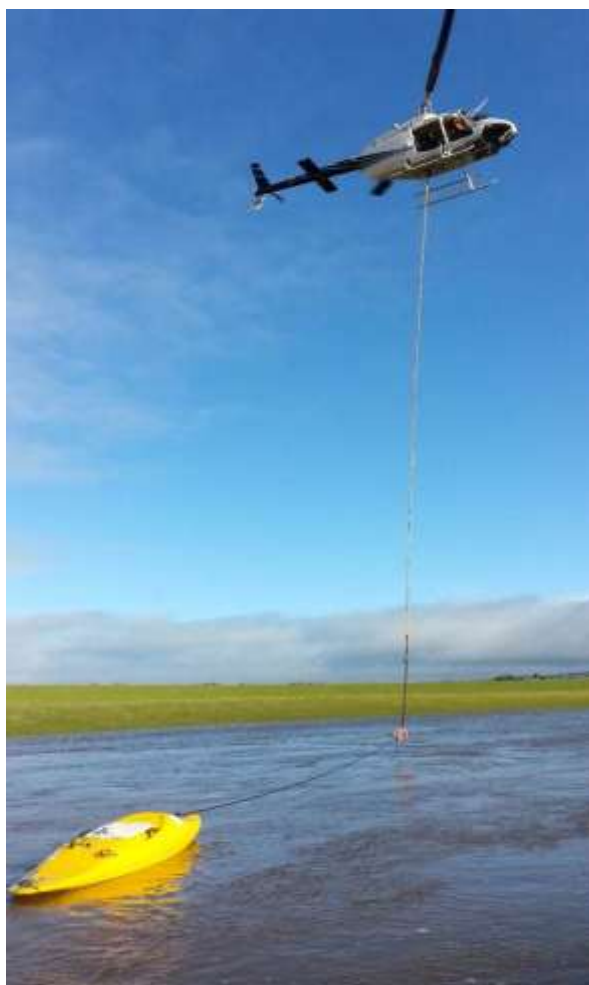
Figure 55. Heli-gauging underway on the Tokomairiro River using a kayak-mounted acoustic Doppler current profiler (ADCP) flow-measuring device
